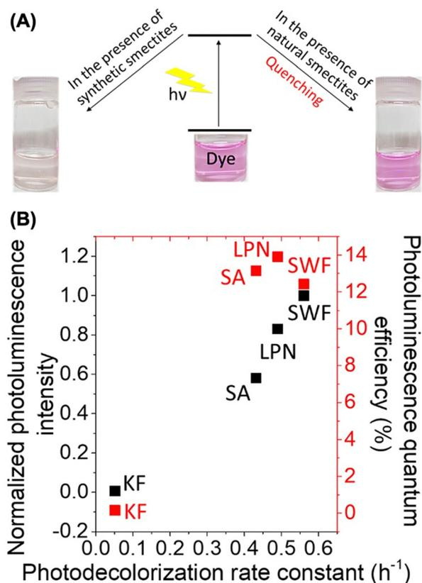
Fig. 19 (A) Photograph of an organic luminophore (Rhodamine 6G) and (B) relationship of the photodecolorisation rate constant with the normalised photoluminescence intensity (black) and the photoluminescence quantum efficiency (red) of SWF-R6G, SA-R6G, LPN-R6G, and KF-R6G suspensions.<sup>396</sup>
