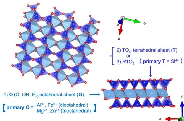
Fig. 14 Structure of a 2:1-type phyllosilicate, two  $\text{TO}_4$  (the primary element of  $\text{T} = \text{Si}^{4+}$ ) tetrahedral sheets (T) on each side of an  $\text{O}$  (O, OH, F) octahedral sheet (O) occupied by octahedrally coordinated cations (e.g.,  $\text{Mg}^{2+}$ ,  $\text{Zn}^{2+}/\text{Al}^{3+}$ ,  $\text{Fe}^{3+}$ , etc.), forming a T–O–T layer (prepared using VESTA software).<sup>44</sup>
