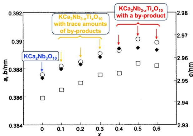
Fig. 35 Variation in the lattice parameters of  $\text{KCa}_2\text{Nb}_{3-x}\text{Ti}_x\text{O}_{10}$  by isomorphous substitution, where an increase in the lattice parameters of  $\text{KCa}_2\text{Nb}_{3-x}\text{Ti}_x\text{O}_{10}$  are correlated with  $x$ , according to Vegard's law.<sup>554</sup>
