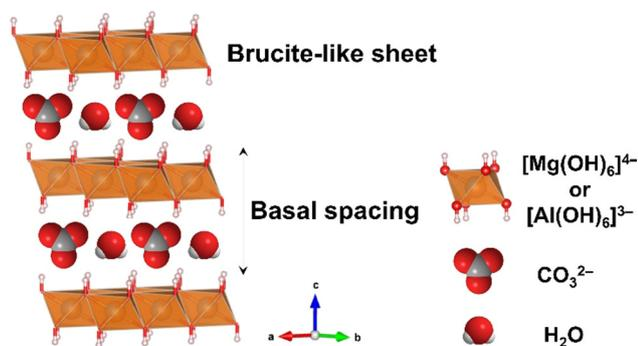
Fig. 4 Structure of layered double hydroxides. The crystal structure was drawn using the VESTA program.<sup>44</sup>
