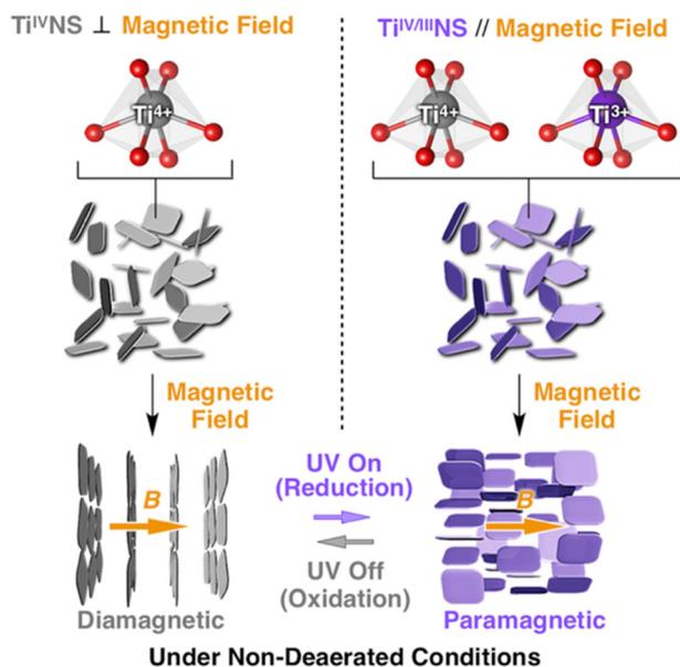
Fig. 28 Schematics of the magnetic orientation;  $\text{Ti}^{4+}$ -based nanosheet ( $\text{Ti}^{\text{IV}}\text{NS}$ ; left) and its reduced form containing  $\text{Ti}^{3+}$  species ( $\text{Ti}^{\text{IV/III}}\text{NS}$ ; right) orient their 2D planes orthogonal and parallel to the applied magnetic field, respectively. Reprinted from ref. 507. Copyright (2018), the American Chemical Society.
