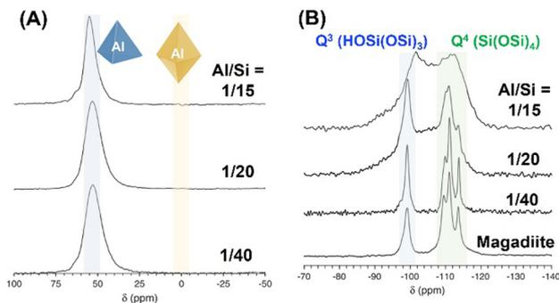
Fig. 13 (A)  $^{27}\text{Al}$  and (B)  $^{29}\text{Si}$  MAS NMR spectra of Al-containing magadiite using aluminium oxyhydroxide.<sup>226</sup>
