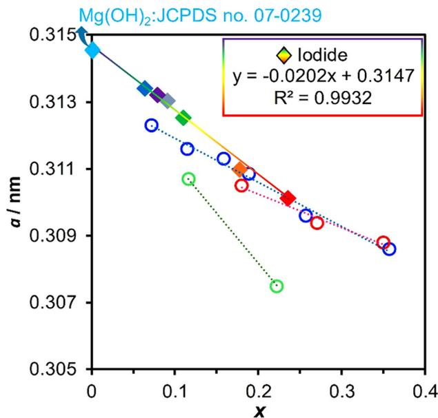
**Fig. 6** Relationships between the lattice parameter  $a$  and composition  $x$  in the reported MgGa-LDHs. Diamonds are for iodide-type MgGa-LDHs<sup>130</sup> and circles are for the carbonate-type MgGa-LDHs.<sup>131–134</sup>
