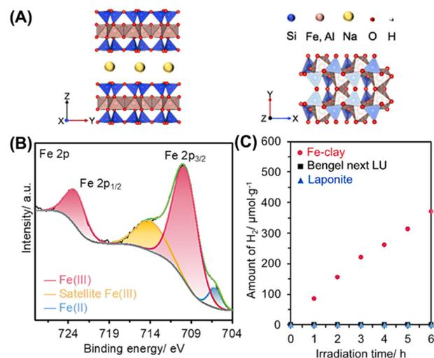
Fig. 20 (A) Polyhedral model of the smectite structure from the [100] direction and [001] direction, (B) Fe 2p XPS spectrum of Fe-clay, and (C) photocatalytic  $\text{H}_2$  evolution of Fe-clay (red circle), Bengel next LU (black square), and LAPONITE<sup>®</sup> (blue triangle) from aqueous MeOH.<sup>386</sup>
