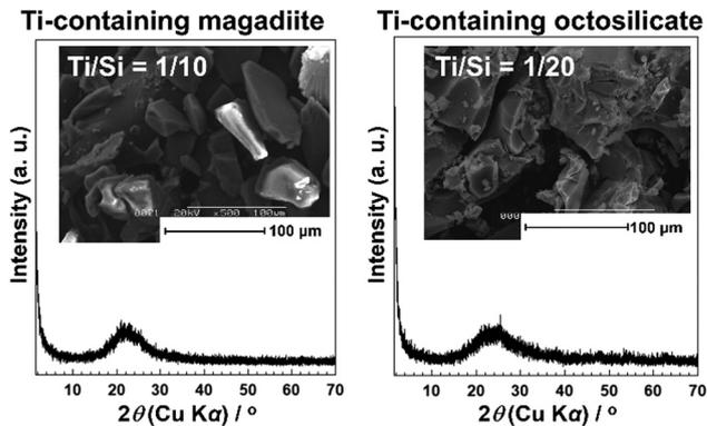
Fig. 10 XRD pattern and SEM image of the Ti-containing magadiites and octosilicates (Ti/Si = 1/10 and 1/20).<sup>245</sup>
