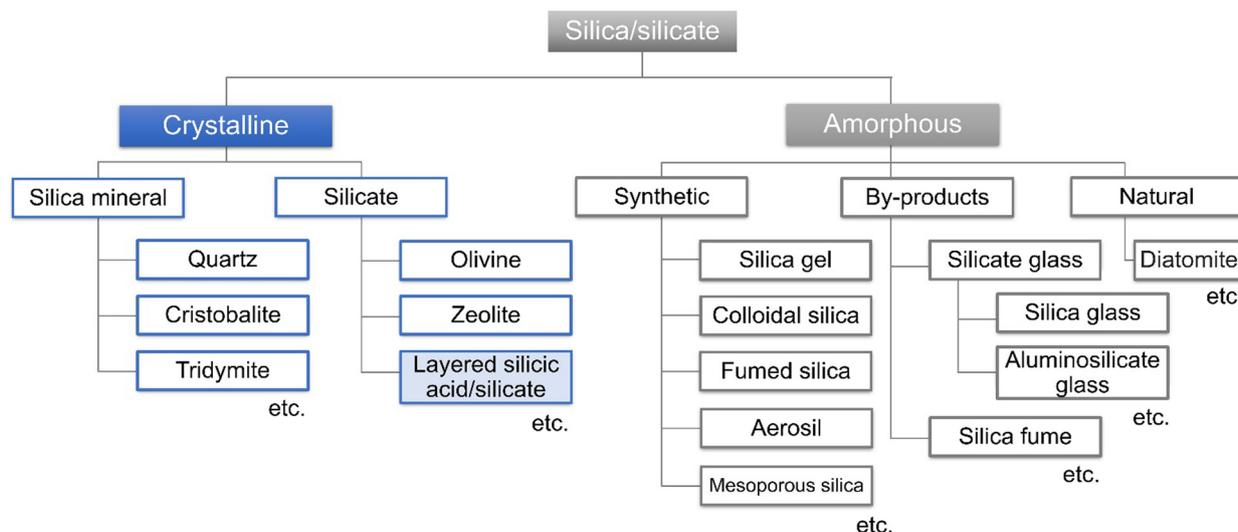
Fig. 8 Classification of crystalline and amorphous silica/silicates.
