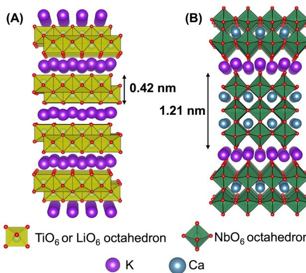
Fig. 30 Crystal structures of (A) lepidocrocite-type layered titanate  $\text{K}_{0.8}\text{Ti}_{1.73}\text{Li}_{0.27}\text{O}_4$  and (B) Dion–Jacobson-type layered perovskite  $\text{KCa}_2\text{Nb}_3\text{O}_{10}$ . The structural parameters were referred from ref. 528 and 529, respectively. The crystal structure was drawn using the VESTA program.<sup>44</sup>
