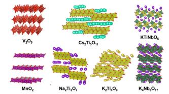
Fig. 27 Variation in LTMOs. 492-498 The crystal structure was drawn using the VESTA program.44
