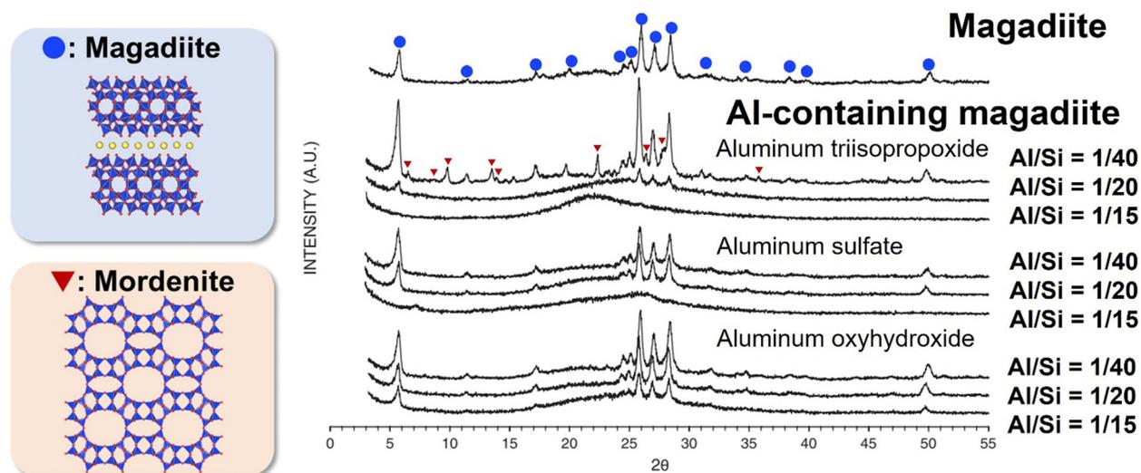
Fig. 12 XRD patterns of magadiite and Al-containing magadiites using aluminium triisopropoxide, aluminium sulfate and aluminium oxyhydroxide (Al/Si = 1/40, 1/20 and 1/15) as the aluminium source.<sup>226</sup>
