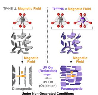
**Fig. 28** Schematics of the magnetic orientation, Ti<sup>4+</sup>-based nanosheet (Ti<sup>IV</sup>NS; left) and its reduced form containing Ti<sup>3+</sup> species (Ti<sup>IV/III</sup>NS; right) orient their 2D planes orthogonal and parallel to the applied magnetic field, respectively. Reprinted from ref. 507. Copyright (2018), the American Chemical Society.
