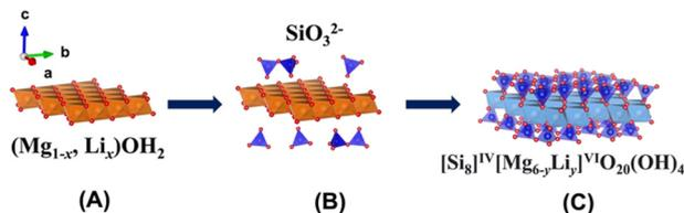
Fig. 21 Route for the formation of hectorite: (A) substitution or fixation of Li into brucite  $\text{Mg}(\text{OH})_2$  sheet, (B) adsorption of silicate anions on the octahedral sheet and (C) progress of the silicate anions to form the 2:1 type phyllosilicate.<sup>427</sup>
