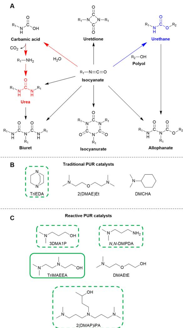
**Fig. 10** (A) Overview of possible polymerization reactions in the synthesis of polyurethane. The two primary polymerization reactions, namely gelling (urethane formation) and blowing (urea formation) are highlighted in blue and red, respectively. Examples of (B) traditional PUR catalysts and (C) novel reactive PUR catalysts which have been (green frame) or could potentially be (green dashed frame) produced from (hemi)cellulose-derived oxygenates.
