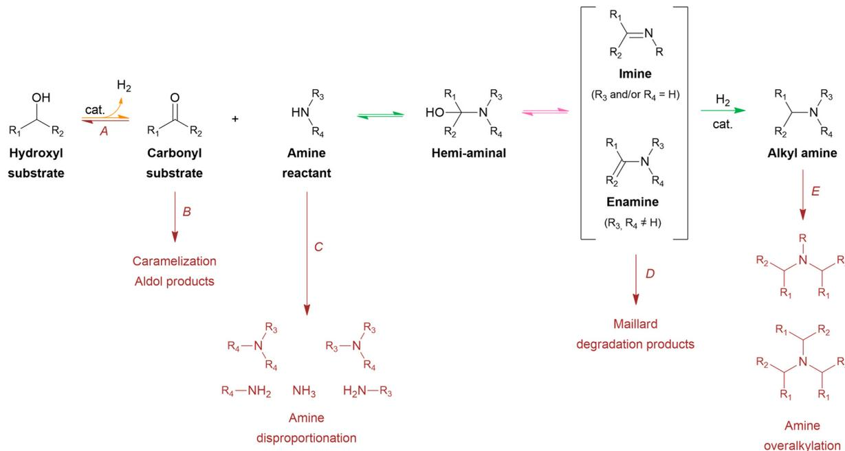
**Scheme 2** General mechanism of the reductive amination of an oxygenate into an alkyl amine. Each elementary reaction is represented by a color; amination (green), dehydration (pink) and (de)hydrogenation (orange). Reactions in dark red represent the most important side reactions.
