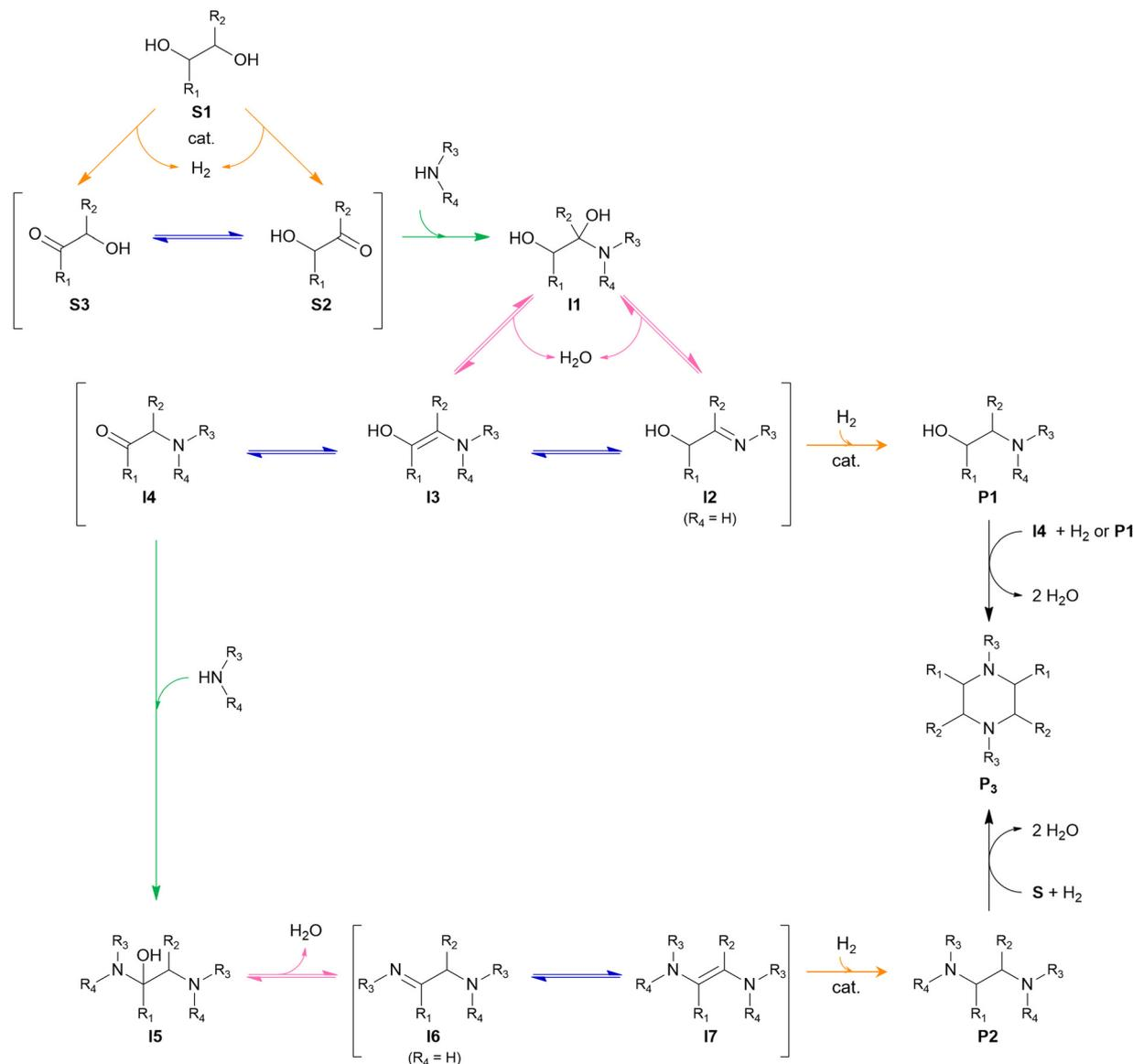
**Scheme 4** General reaction mechanism of the reductive amination of O<sub>2</sub> substrates. Each elementary key reaction is represented by a color: amination (green), isomerization (blue), dehydration (pink), and (de)hydrogenation (orange).
