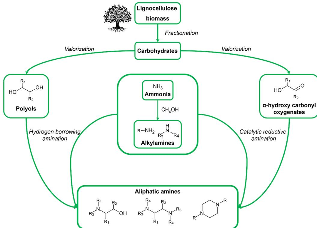
Fig. 13 Schematic overview of the holistic aliphatic amine industry. The carbon part of the aliphatic amines originates from oxygenates obtained via valorization of lignocellulose-derived carbohydrates. The nitrogen part originates from green ammonia and bio-alcohol-derived alkylamines.
