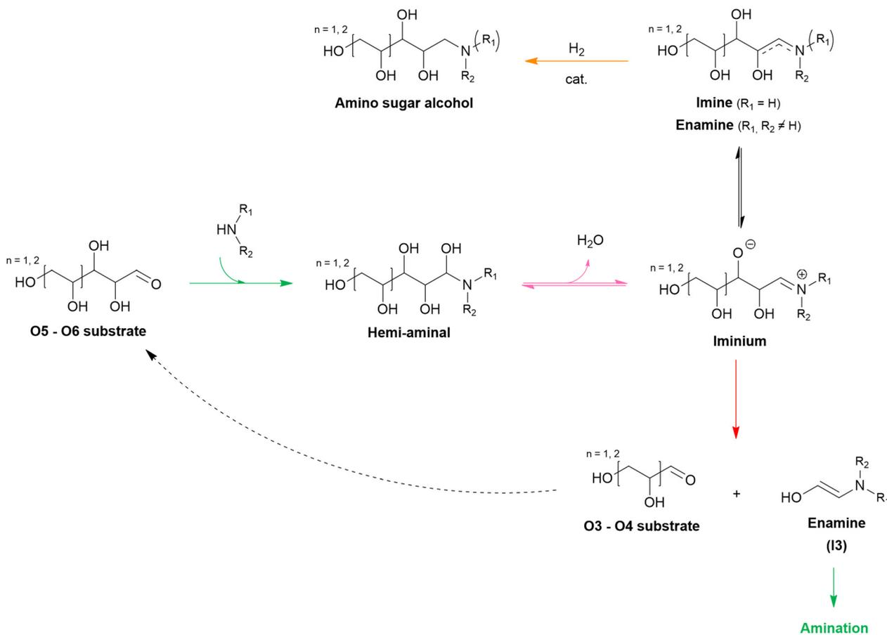
**Scheme 6** General reaction mechanism of the reductive amination of **O5** and **O6** substrates. Each elementary key reaction is represented by a color: amination (green), retro-aldol condensation (red), dehydration (pink) and (de)hydrogenation (orange).
