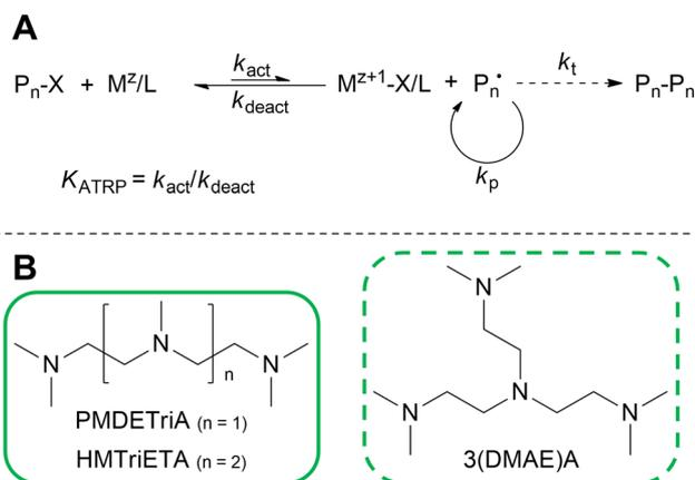
**Fig. 11** (A) General principles of atom transfer radical polymerization. (B) Examples of ATRP catalytic ligands which have been (green frame) or could potentially be (green dashed frame) produced from (hemi)cellulose-derived oxygenates.
