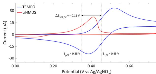
**Fig. 9** CVs of TEMPO and LiHMDS in *o*-difluorobenzene with [t<sup>o</sup>Bu<sub>4</sub>N][PF<sub>6</sub>] (0.2 M) as supporting electrolyte at a scan rate of 100 mV s<sup>-1</sup>, showing an irreversible and reversible redox event, respectively. For clarity, the CVs are shown partly. The full spectra and experimental details are reported in the ESI.†  $E_{1/2}$  (Fc/Fc<sup>+</sup>) = +0.22 V vs. Ag/AgNO<sub>3</sub>.
