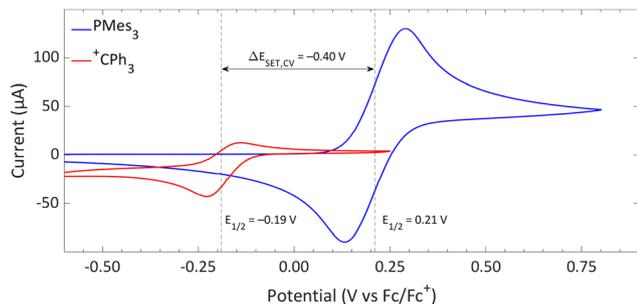
Fig. 1 CVs of  $\text{PMes}_3$  and  $[\text{CPh}_3][\text{B}(\text{C}_6\text{F}_5)_4]$  in DCM with  $[\text{nBu}_4\text{N}][\text{PF}_6]$  (0.5 M) as electrolyte at a scan rate of  $100 \text{ mV s}^{-1}$ , showing a quasi-reversible and reversible redox event, respectively. Further experimental details are reported in the ESI.†
