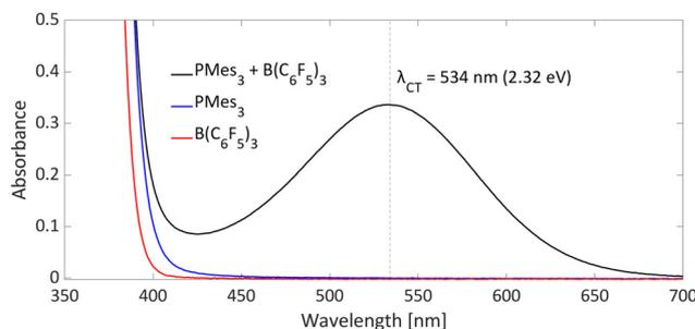
Fig. 4 UV-vis spectrum of toluene solutions of  $\text{PMes}_3$  (45 mM; blue),  $\text{B}(\text{C}_6\text{F}_5)_3$  (30 mM; red) and the combination of  $\text{PMes}_3$  (45 mM) and  $\text{B}(\text{C}_6\text{F}_5)_3$  (30 mM; in black).
