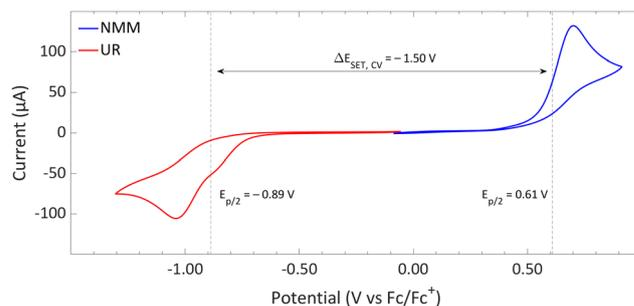
**Fig. 14** CVs of Umemoto's reagent (UR) and NMM in acetonitrile using [nBu<sub>4</sub>N][BF<sub>4</sub>] (0.5 M) as supporting electrolyte at a scan rate of 100 mV s<sup>-1</sup>, showing irreversible redox events for both. Experimental details are reported in the ESI.†
