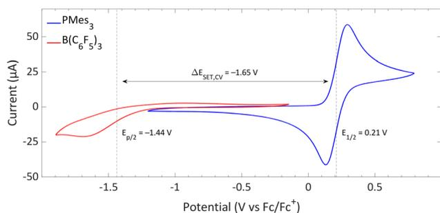
Fig. 2 CVs of  $\text{B}(\text{C}_6\text{F}_5)_3$  and  $\text{PMes}_3$  in DCM at a scan rate of  $100 \text{ mV s}^{-1}$ , showing an irreversible and reversible redox event, respectively. For  $\text{B}(\text{C}_6\text{F}_5)_3$ ,  $[\text{nBu}_4\text{N}][\text{B}(\text{C}_6\text{F}_5)_4]$  (0.05 M) was used as electrolyte, while for  $\text{PMes}_3$   $[\text{nBu}_4\text{N}][\text{PF}_6]$  (0.5 M) was used. Experimental details are reported in the ESI.†
