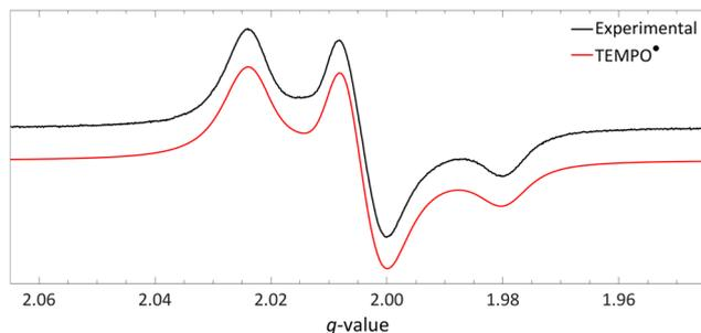
**Fig. 10** Obtained EPR spectrum of a flash frozen solution of LiHMDS and [TEMPO][BF<sub>4</sub>] to yield TEMPO\* ( $g_{\perp} = 2.0067$ ,  $g_{\parallel} = 2.0014$ ,  $^{14}\text{N}a_{\perp} = 0.77$  mT and  $^{14}\text{N}a_{\parallel} = 3.7$  mT) in PhCF<sub>3</sub>. Further experimental and simulation details are reported in the ESI.†
