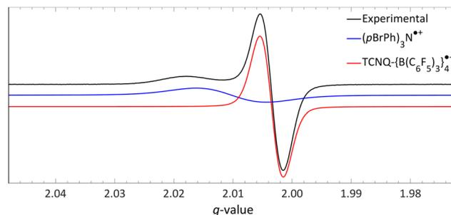
**Fig. 13** Room temperature EPR of the combination of  $\text{TCNQ}\{-\text{B}(\text{C}_6\text{F}_5)_3\}_4$  ( $g_{\text{iso}} = 2.0035$ ) and  $(p\text{BrPh})_3\text{N}$  ( $g_{\text{iso}} = 2.0103$ ) in DCM. Further experimental and simulation details are reported in the ESI.†
