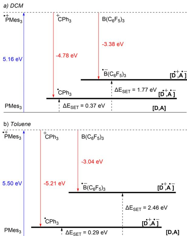
Fig. 3 Energy diagram with calculated ionisation energy (IE) of  $\text{PMes}_3$  (blue) and electron affinities (EA) of  $\text{CPh}_3^+$  and  $\text{B}(\text{C}_6\text{F}_5)_3$  (both red) for both (a) DCM and (b) toluene as the solvent. For both the photoinduced SET ( $\text{PMes}_3, \text{B}(\text{C}_6\text{F}_5)_3$ ) and thermally induced SET ( $\text{PMes}_3, \text{CPh}_3^+$ ) the  $\Delta E_{\text{SET,calc}}$  are indicated (black arrows).
