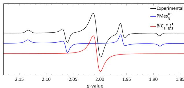
Fig. 6 A 30 K EPR spectrum of  $\text{PMes}_3$  and  $\text{B}(\text{C}_6\text{F}_5)_3$  using 390–500 nm irradiation yielding photoinduced SET to afford the RIP consisting of  $\text{PMes}_3^{\bullet+}$  ( $g_{\perp} = 2.0050$ ,  $g_{\parallel} = 2.0022$ ,  $^{31}\text{P}a_{\perp} = 17.0$  mT,  $^{31}\text{P}a_{\parallel} = 41.0$  mT) and  $\text{B}(\text{C}_6\text{F}_5)_3^{\bullet-}$  ( $g_{\text{iso}} = 2.0057$ ). Further experimental and simulation details are reported in the ESI.†
