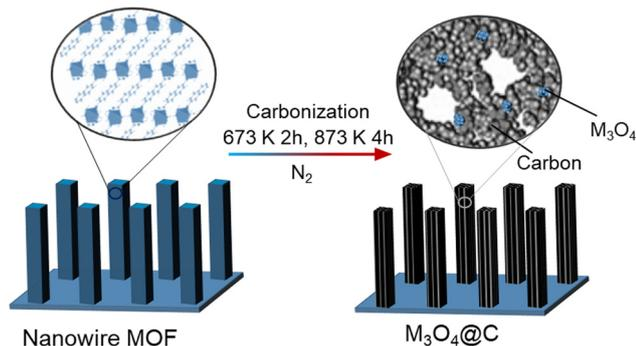
Fig. 5 Schematic illustration for the fabrication of  $M_3O_4$ -C nanowire arrays.<sup>92</sup> Inspired from ref. 92.
