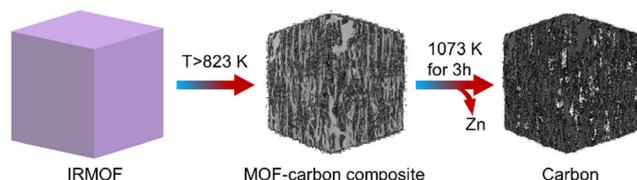
Fig. 3 Schematic depiction of the structural changes of IRMOF-1 with heat treatment to yield MDC-1.<sup>37</sup>
