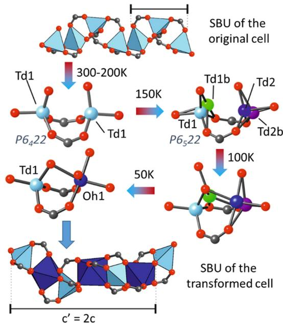
**Fig. 12** Schematic depiction of the structural transition occurring in the  $[\text{Zn}_{0.79}\text{Co}_{0.21}(\text{hfipbb})]$  material upon cooling. The inorganic SBU might adapt to include octahedrally coordinated cations, which results in a unit cell transformation with a doubled  $c$  parameter.<sup>195</sup> Image modified with permission of Science.
