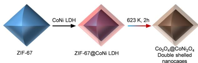
**Fig. 4** Schematic illustration of the formation process of Co<sub>3</sub>O<sub>4</sub>@NiCo<sub>2</sub>O<sub>4</sub> double-shelled nanocages.<sup>87</sup>
