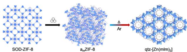
Fig. 8 Schematic depiction of the synthetic approach to obtain a new **qtz**-topology from a mechanically amorphised ZIF.<sup>153</sup> Reproduced from ref. 153 with permission from Royal Chemical Society, copyright 2022.
