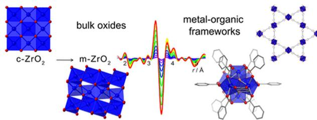
Fig. 15 Schematic depiction of the metal-node phase transition of NU-1000 and UiO-66 structures upon heating.<sup>208</sup> Reproduced from ref. 208 with permission from American Chemical Society, copyright 2017.
