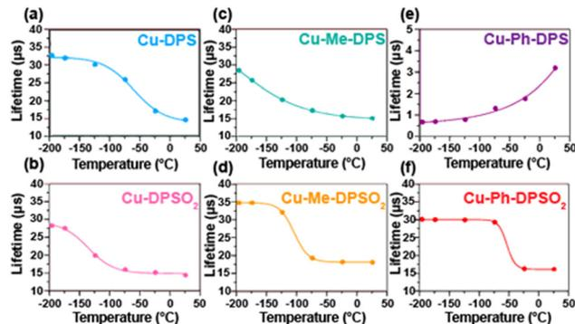
Fig. 6 Solid-state photoluminescence lifetimes of (a) Cu-DPS; (b) Cu-DPSO<sub>2</sub>; (c) Cu-Me-DPS; (d) Cu-Me-DPSO<sub>2</sub>; (e) Cu-Ph-DPS; and (f) Cu-Ph-DPSO<sub>2</sub> from –196 to 25 °C. Samples drop-cast as neat thin-films from MeOH on quartz slides ( $\lambda_{\text{exc}} = 370$  nm). Reproduced from ref. 173. Copyright 2019, American Chemical Society.
