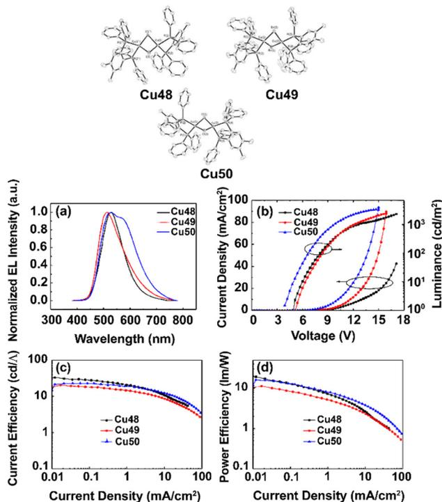
Fig. 31 ORTEP diagrams of complexes **Cu48–50**. (a) Electroluminescence spectra of devices **Cu48–50**; (b) current density–voltage–luminance characteristics ( $J$ – $V$ – $L$ ) of devices **17–A3**; (c) EQE versus current density curves for devices **Cu48–50**; (d) power efficiency versus current density for devices **Cu48–50**. Reproduced with permissions from ref. 323. Copyright 2016, Elsevier.
