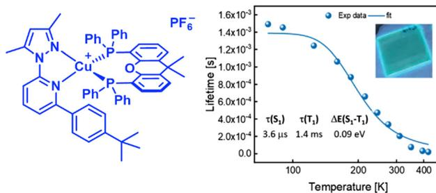
Fig. 13 Left: Structural representation of a highly emissive blue-emitting Cu(I) complex. Right:  $\langle \tau \rangle$  vs. temperature plot the corresponding thin-film fitted with eqn (6), thin-film under UV irradiation ( $\lambda_{\text{ex}} = 305 \text{ nm}$ ) is depicted as inset. Reproduced with permission from ref. 228.
