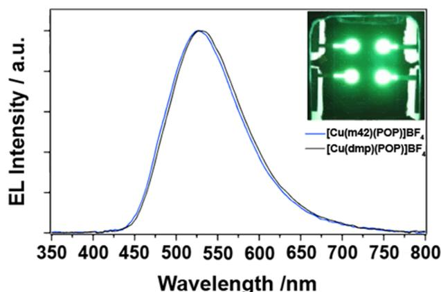
Fig. 33 Electroluminescence spectra at 10 V of OLEDs based on **Cu66** and **Cu4**. In the inset is reported a photograph of OLEDs based on **Cu66**. Reproduced with permissions from ref. 238. Copyright 2018, American Chemical Society.
