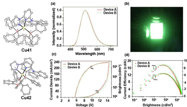
Fig. 30 ORTEP diagrams of **Cu41** and **Cu42** with thermal ellipsoids at 30% probability level. Solvent molecules, the anion, and H atoms are omitted for clarity. (a) Electroluminescence spectra (device a = **Cu41**, device b = **Cu42**); (b) photo of Device B; (c) current density–voltage–brightness ( $I$ – $V$ – $B$ ) curves; (d) plots of EQE and current efficiency vs. brightness. Reproduced with permissions from ref. 320. Copyright 2015, Royal Society of Chemistry.
