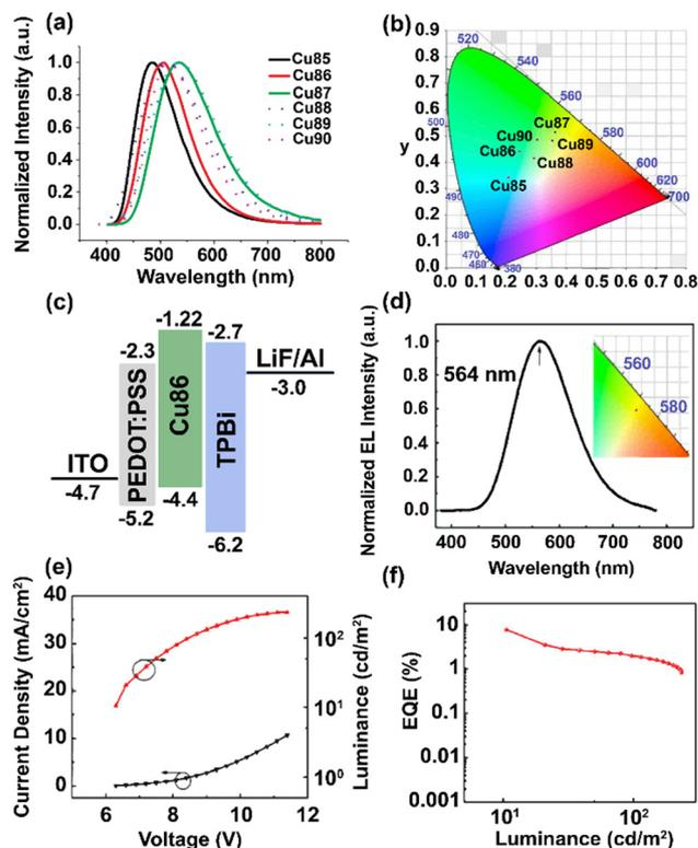
Fig. 36 (a) Normalized emission spectra and (b) CIE graph of complexes **Cu85–90** in powder state at 297 K. Reproduced from ref. 334. (c) Energy-level diagram of the device based on the complex **Cu86**; (d) electroluminescence spectra, and the inset is the CIE of electroluminescence spectra; (e) current density–voltage–luminance ( $J$ – $V$ – $L$ ) characteristics; (f) EQE–luminance characteristics. Reproduced from ref. 334. Copyright 2020, Elsevier.
