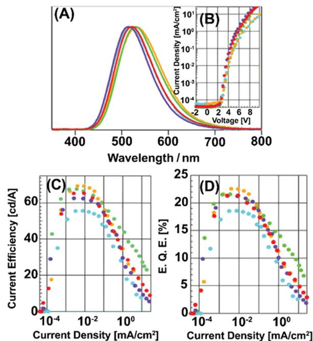
Fig. 29 Properties of OLEDs containing complex **Cu34** (green line), complex **Cu35** (red line), complex **Cu36** (purple line), complex **Cu37** (orange line) and complex **Cu38** (blue line). (A) Electroluminescence spectra; (B) the dependence of the EQE on the current density; (C)  $I$ - $V$  characteristics; (D) the dependence of the current efficiency on the current density. Reproduced with permissions from ref. 319. Copyright 2015, Royal Society of Chemistry.
