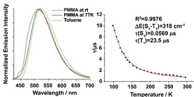
Fig. 27 Emission spectra and lifetime data of **Au49**. (left) Emission spectra of the complex (4 wt%) in PMMA thin-film at rt and 77 K, and in toluene at rt. (right) Plot of emission lifetime monitored at 517 nm against temperature and fitting of the data (red line) to the equation for TADF. Reproduced with permissions from ref. 310. Copyright 2017, Wiley-VCH.
