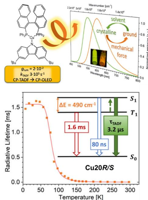
Fig. 16 Top: Structural presentation of **Cu20R/S** and the corresponding emission spectrum of the crystalline and ground powder sample, as well as their UV irradiation, is shown as inset. Bottom: Temperature dependence of the radiative lifetimes of **Cu20R/S** in the ground solid state and the state diagram visualizing the TADF processes. Reproduced with permission from ref. 251.
