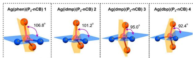
Fig. 20 Coordination core geometries of complexes **Ag1**, **Ag2**, **Ag3** and **Ag4** as found by single-crystal X-ray diffraction analysis. The given interplanar angles characterize the deviations from the tetrahedral geometry ( $\varphi = 90^\circ$ ) (not to be confused with the valence angle of  $109^\circ$  in a tetrahedral molecule such as methane). Represented with permission from ref. 269.
