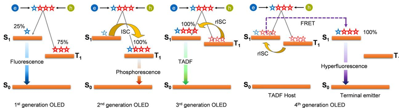
Fig. 4 Sketch of the working principles of 1<sup>st</sup>, 2<sup>nd</sup>, 3<sup>rd</sup>, and 4<sup>th</sup> generation OLEDs. The transition processes of photogenerated excitons for fluorescence, phosphorescence, TADF, and hyperfluorescence are highlighted.
