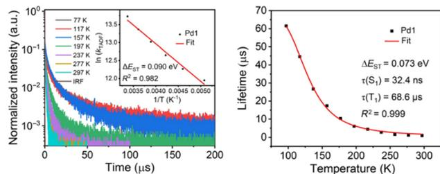
**Fig. 10** Left: Temperature-dependent transient PL characteristics of **Pd1** in PMMA films. Inset: Arrhenius fit of the  $k_{DF}$  value vs. temperature. Right: Boltzmann-type fitting of the emission lifetimes of **Pd1** in PMMA film at various temperatures. Printed with permission from ref. 200.
