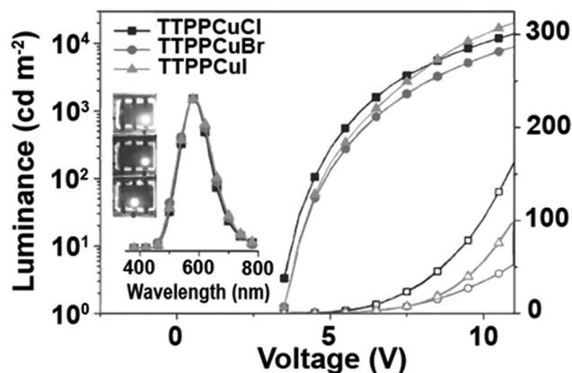
Fig. 32 Electroluminescence performance of TTPPCuX-based OLEDs. Current density ( $J$ ) (hollow)–luminance (solid)–voltage curves, electroluminescence spectra at  $1000 \text{ cd m}^{-2}$  and device photos at 5 V (inset). Reproduced with permissions from ref. 326. Copyright 2016, Europe PMC.
