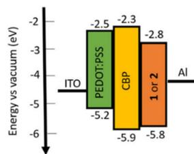
Fig. 38 Energy diagram of the multilayer device architecture (**1** = **Cu108**, **2** = **Cu153**, HOMO and LUMO levels were derived from cyclic voltammetry). Reproduced with permissions from ref. 388.
