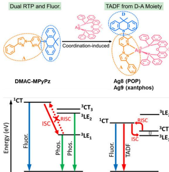
Fig. 22 Top: Molecular design strategies for the realization of TADF including the molecular structure of **Ag8** and **Ag9**. Bottom: PL processes for the free DMAC-MPyPz ligand (left) and the corresponding Ag(I) complexes (right). Printed with permission from ref. 272.
