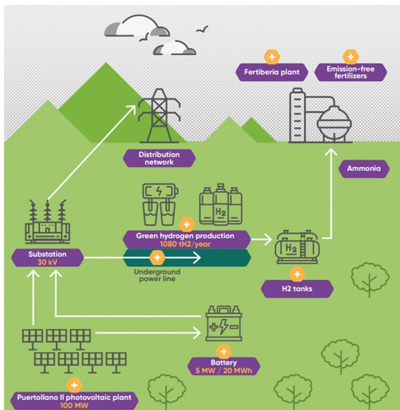
Fig. 19 Schematics of Puertollano ammonia plant. Source: Iberdrola.
