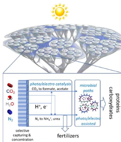
Fig. 18 Schematic representation of an artificial-tree for the local generation of solar fuels and chemicals. Reproduced with permission from Centi *et al.*<sup>356</sup>
