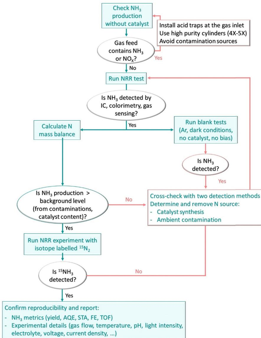
Fig. 15 Suggested protocol for benchmarking light-driven NRR experiments.
