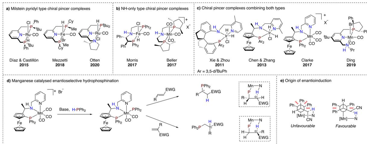
**Scheme 3** (a) Chiral Milstein pyridyl type pincer complexes; (b) chiral NH-only type pincer complexes; (c) chiral pincer complexes with merged structural features of both MLC active pincer types; (d) enantioselective hydrophosphination of  $\alpha,\beta$ -unsaturated compounds catalysed by Clarke's manganese catalyst; (e) proposed origin of enantioinduction for the manganese catalysed enantioselective hydrophosphination.
