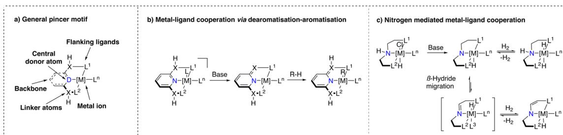
**Scheme 2** (a) General pincer complex structure; (b) base induced dearomatisation–aromatisation MLC activation mode of Milstein pyridyl type pincer complexes; (c) base induced MLC activation modes of NH-only type pincer complexes.
