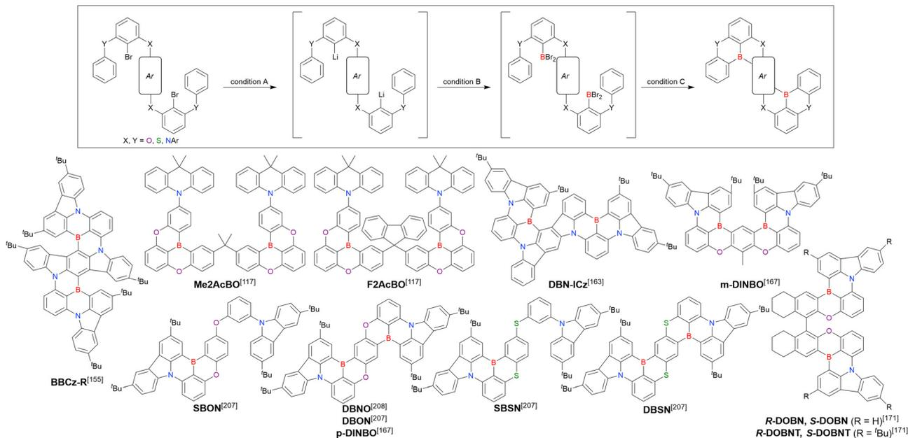
Fig. 18 MR-TADF emitters synthesised by one-pot double borylation.
