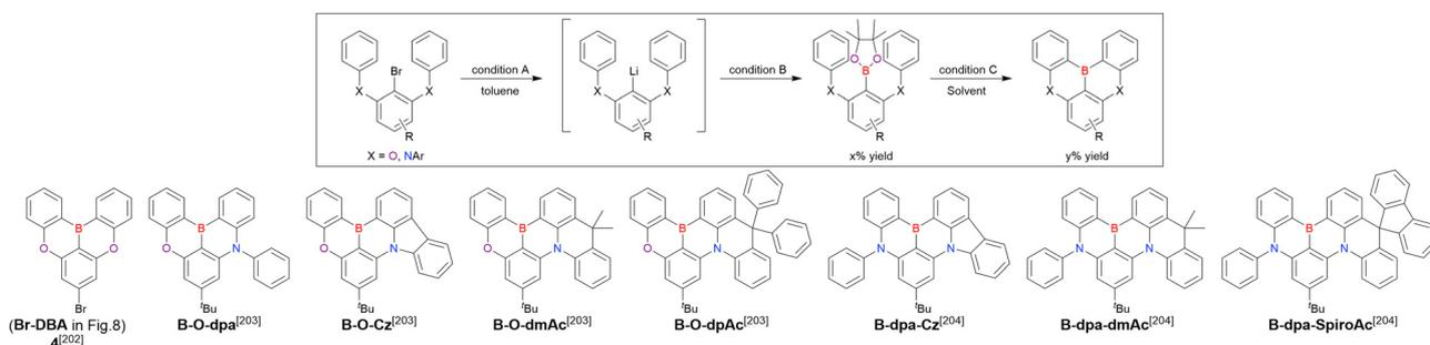
Fig. 16 MR-TADF emitters synthesised by stepwise borylation-cyclisation.
