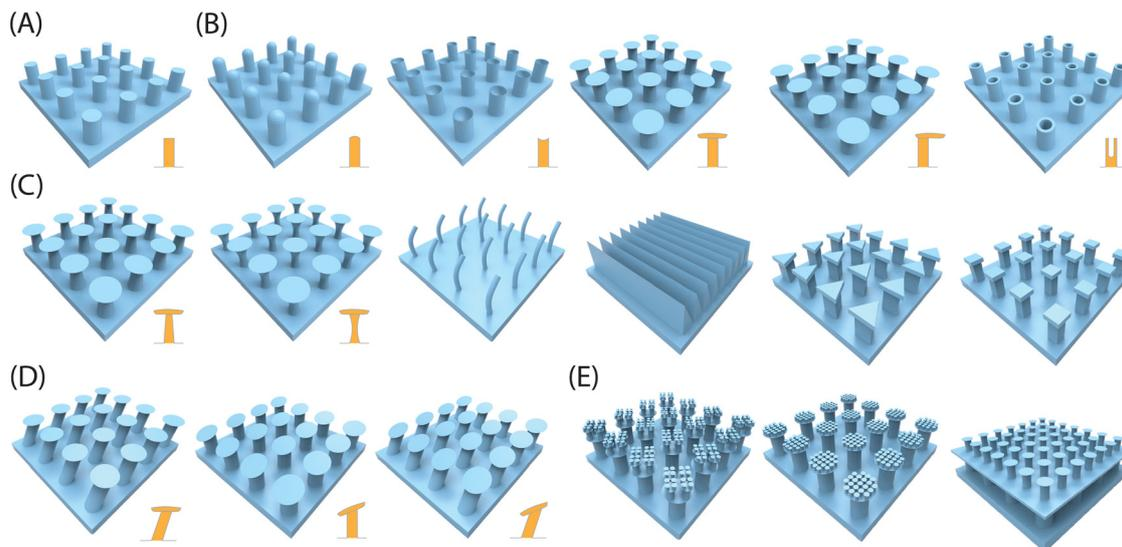
**Fig. 12** The development of gecko-inspired dry adhesive structures. (A) Vertically aligned micro- and nanofibers. (B) Tips with different shapes. (C) Fibril stems with different shapes. (D) Anisotropic structures, including fibril sloping stems, sloping tips, and a combination of both. (E) Hierarchical structures.
