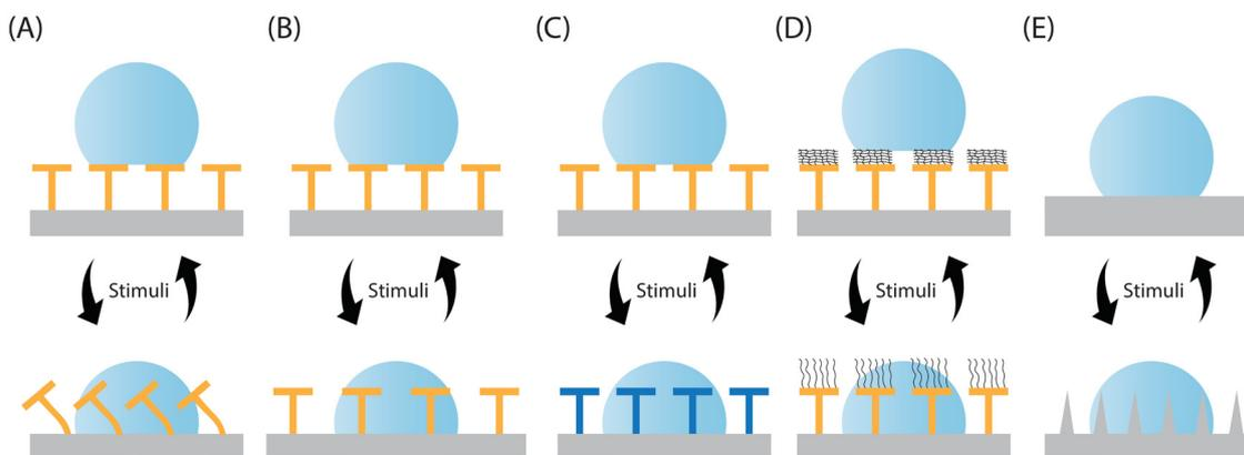
**Fig. 18** Construction strategies to control surface wetting and adhesion for solid structure surfaces. (A) Modulating the physical shape of micro-nano structures. (B) Modulating the distribution and morphology of micro-nanostructures on the surface through stretching or bending of the substrate. (C) Modulating the chemical properties of micro-nano structures. (D) Modulating the acting state of functional molecules. (E) Modulating the formation or disappearance of microneedles.
