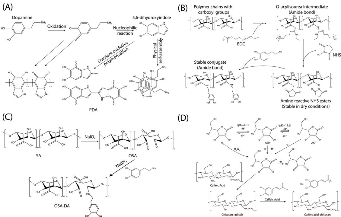
**Fig. 10** Schematics of typical modification methods for incorporating catechol and its derivatives into polymers. (A) Self-polymerization of dopamine. (B) 1-Ethyl-3-(3-dimethylaminopropyl) carbodiimide/*N*-hydroxysuccinimide (EDC/NHS) coupling chemistry. (C) Schiff-base chemistry. (D) The free radical-induced grafting method using the ascorbic acid/ $\text{H}_2\text{O}_2$  redox system.
