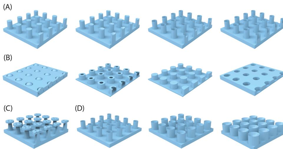
**Fig. 14** The development of octopus-inspired wet adhesive structures. (A) Suckers with different curvature radii ( $\sim 1.00$ ,  $\sim 0.66$ ,  $\sim 0.84$ ,  $\sim 0.93$ ). (B) Suckers with different shapes, including octopus-inspired architecture, perforated cylinders, cylindrical pillars and cylindrical holes. (C) Hierarchical micropillars with suckers on top. (D) Suckers with different diameter sizes (15, 50, and 500  $\mu\text{m}$  in diameter) with  $\sim 0.93$  curvature.
