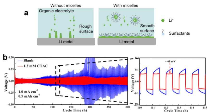
Fig. 15 (a) Scheme of inhibition of Li dendrite in lithium–ion batteries. (b) Cycling performance in symmetric cells, without or with CTAC additives, at current densities of  $1.0 \text{ mA cm}^{-2}$  with a fixed capacity of  $0.5 \text{ mA h cm}^{-2}$ . Enlarged figures on the right show detailed voltage profiles with cycle time indicated. Image adapted from ref. 173 with permission from American Chemical Society, copyright 2018.
