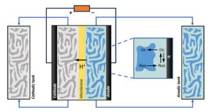
Fig. 17 General scheme of a RFB with bicontinuous microemulsion electrolytes. Redox reactions are shown in the oil phase (inset). Water phase: light grey (cathode), light blue (anode); oil phase: dark grey (cathode), dark blue (anode). 185
