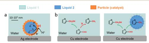
Fig. 14 (a) Schematic illustration of ECH of styrene in particle-stabilised emulsions. 142 (b) Schematic representation of emulsion-promoted EC-HDO of FF. 145
