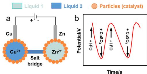
Fig. 8 (a) Sketch of liquid marble micro-Daniell cell.<sup>118</sup> (b) Potential variation in liquid marble Daniell cell through the entire pumping process of two cycles.
