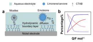
Fig. 13 (a) Solubilisation equilibria and substrate diffusion of D-limonene and carvone to the electrode in micellar and emulsified solutions. (b) Relative percentage of D-limonene, p-menthene and p-menthane for ECH in hydroorganic solutions. 142,143 blue: with micellar solution, red: without micellar solution; dash-line: reactants, solid-line: products.
