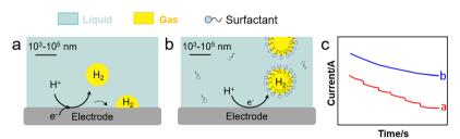
Fig. 9 HER on an electrode (a) before and (b) after electrolyte modification with a surfactant (e.g., CTAB), and (c) current response of applied potential from open-circuit to -1.0 V vs. Ag/AgCl in  $H_2SO_4$  with (blue) and without (red) CTAB (0.1 g  $L^{-1}$ ).
