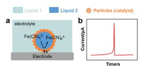
Fig. 7 (a) Scheme of an EDR experiment for a particle-stabilised droplet interacting with an electrode. 114 (b) Chronoamperometric curve from EDR experiment with spike signals corresponding to the charge transfer of a Pickering emulsion.
