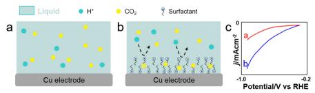
Fig. 12 Scheme showing CO<sub>2</sub> and H<sup>+</sup> transfer from the bulk electrolyte to the electrode surface. (a) and (b) With/without surfactant on Cu nanowires. (c) Linear sweep voltammetry (LSV) of Cu nanowire electrodes with/without CTAC modification in the CO<sub>2</sub>-saturated 0.1 m KHCO<sub>3</sub> aqueous solution. 136
