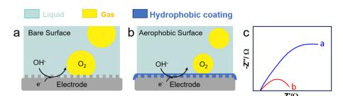
Fig. 10 OER on an electrode (a) before and (b) after modification with a surfactant (e.g., CTAB), and (c) EIS response with (blue) and without (red) CTAB (0.1 a  $L^{-1}$ ). 122
