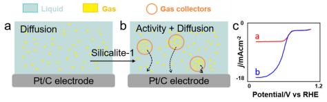
Fig. 11 ORR conducted (a) without and (b) with silicalite-1 nanocapsules (NCs) (red circles) working as gas collectors to transport O<sub>2</sub> (yellow) in water (blue) to the electrode surface. (c) RDE voltammograms collected for O2-saturated phosphate-buffered water (0.5 M) solutions at pH 7.0 containing  $0 \text{ mg mL}^{-1}$  (red) and  $122.7 \text{ mg mL}^{-1}$  (blue) of silicalite-1-NCs at a scan rate of  $5 \text{ mV s}^{-1}$  and an electrode rotation rate of 1600 rpm.  $^{132}$
