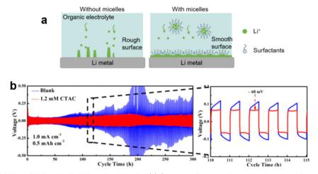
Fig. 15 (a) Scheme of inhibition of Li dendrite in lithium-ion batteries. (b) Cycling performance in symmetric cells, without or with CTAC additives, at current densities of 1.0 mA cm<sup>-2</sup> with a fixed capacity of 0.5 mA h cm<sup>-2</sup>. Enlarged figures on the right show detailed voltage profiles with cycle time indicated. Image adapted from ref. 173 with permission from American Chemical Society, copyright 2018
