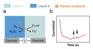
Fig. 5 (a) O2 reduction using Pt nanoparticles and Fc as a sacrificial electron donor at a water–DCE interface. 111 (b) Current spikes in chronoamperometric tests for charge transfer from oil to water.
