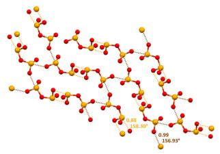
Fig. 4 Partial representation (ball and stick, Mercury 2022.1.0) of the 2D net assembled via ChBs in a salt between diprotonated diazabicylooctane and diselenite dianion (Refcode BOGWEG).<sup>29</sup> Short and long ChBs are ocher and brown dotted lines; ChB angles and Nc values are reported close to the interactions. Colour code: red, oxygen and orange, selenium.
