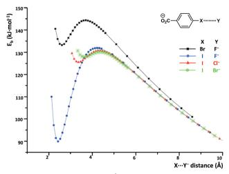
Fig. 3 Binding energy ( $E_{\rm b}$ , kJ mol<sup>-1</sup>) vs. Br/I···halide anion distance of 4-bromo- and 4-iodo-benzoate complexes in the gas phase.<sup>62</sup>
