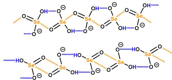
Scheme 1 Infinite chains formed by  $\text{HSeO}_3^-$  anions under synergistic action of ChBs and HBs.<sup>29</sup>
