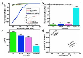
Fig. 17 (a) Linear sweep voltammetry (LSV) curves, (b) current density at -0.6 V, (c) overpotential ( $\eta$ , in mV), and (d) Tafel slope measurements for the hydrogen evolution reaction (HER) for Ni, Ni/Cys (cysteine), Ni/Au, and Ni/Au/Cys films at pH 11 and room temperature, using an Ag wire as the reference, in 0.1 M KOH at a sweep rate of 10 mV s<sup>-1</sup>. Adapted with permission from ref. 137, Copyright 2022, Elsevier.
