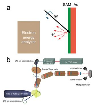
(a) Illustration of the LEPET (low energy photo-electron transmission) photoemission setup used to measure electron energy distributions across chiral monolayers, without the spin of transmitted electron determination. (b) Diagram depicting the experimental setup purposely designed to measure the spin polarization of photoelectrons. Adapted with permission from ref. 21, Copyright 2012, American Chemical Society.
