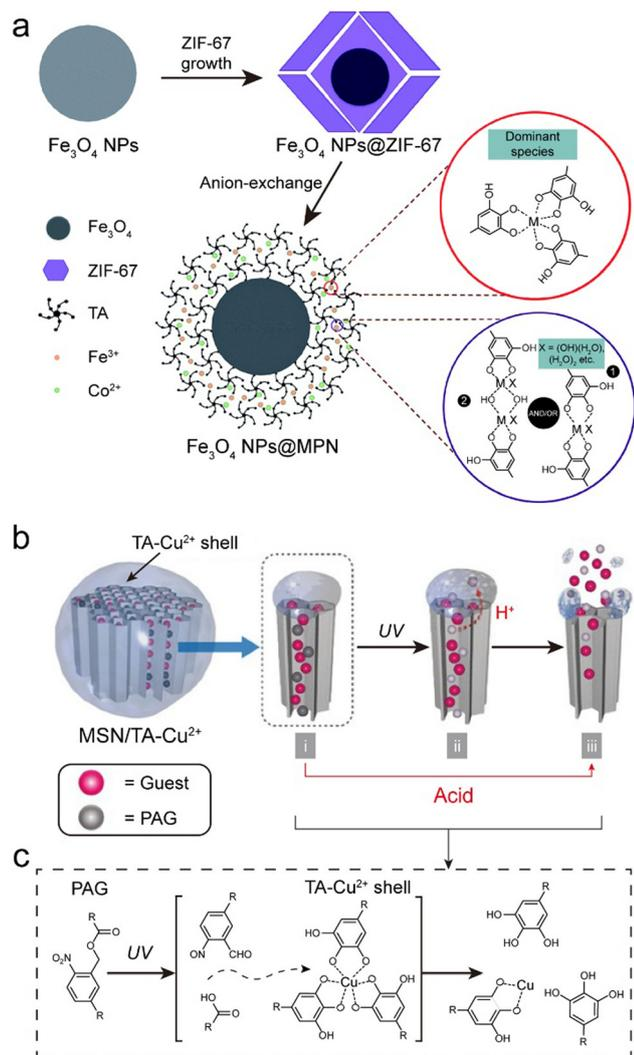
Fig. 17 (a) Schematic illustration of the synthesis of  $\text{Fe}_3\text{O}_4$ @MPN composites. Adapted with permission from ref. 154. Copyright 2019, Royal Society of Chemistry. (b) and (c) Gating activity and adhesion of TA and TA- $\text{Cu}^{2+}$  complexes on the surface of MSN. (b) Schematic and (c) mechanism of decomposition of MPNs ( $\text{Cu}^{2+}$ -TA) by photoacid generators (PAGs) in MPN-MSN composites. (b) and (c) Adapted with permission from ref. 155. Copyright 2017, Wiley-VCH.
