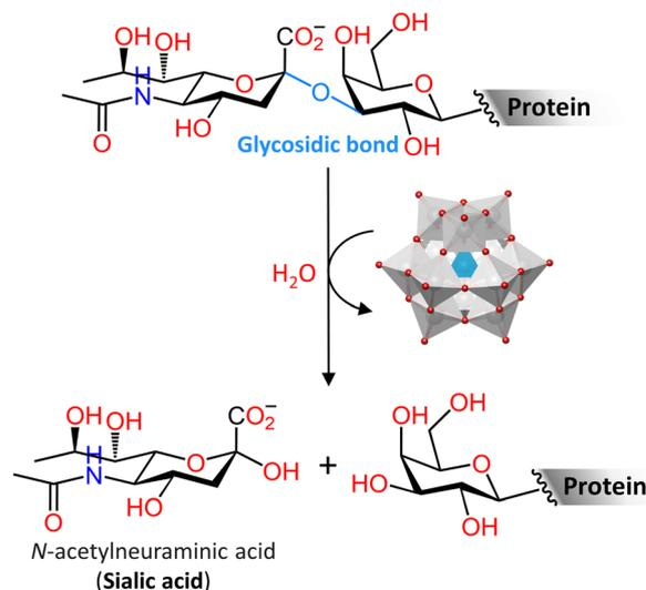
Fig. 15 Hydrolysis of the terminal glycosidic bond of an example glycan chain of a glycoprotein resulting in the release of a sialic acid catalyzed by  $\text{M}_3[\text{EA}_{12}\text{O}_{40}]^{3-}$  ( $\text{M} = \text{H}^+, \text{Na}^+, \text{or K}^+$ ;  $\text{E} = \text{P}^{5+} \text{ or Si}^{4+}$ ;  $\text{A} = \text{W}^{6+} \text{ or Mo}^{6+}$ ).
