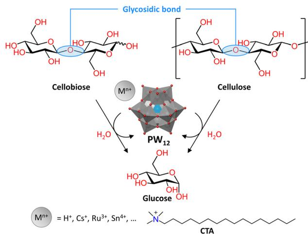
Fig. 12 Hydrolysis of the glycosidic bond in cellobiose and cellulose into glucose catalyzed by  $(\text{M}^{n+})_3/[\text{PW}_{12}\text{O}_{40}]^{3-}$  ( $\text{PW}_{12}$ ) with different counter-ions.
