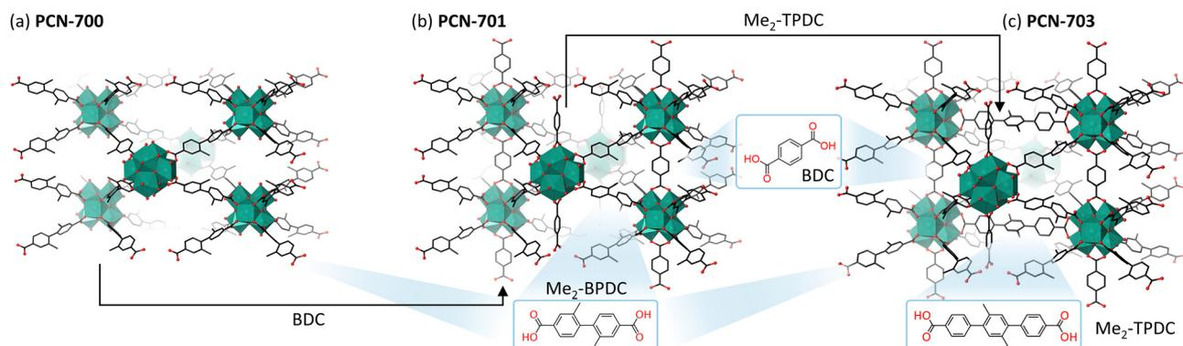
Fig. 22 Structures of MOFs (a) PCN-700, (b) PCN-701, and (c) PCN-703, which differ in terms of the linkers connecting the {Zr<sub>6</sub>O<sub>8</sub>} clusters.
