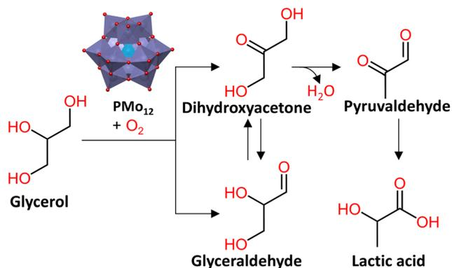
Fig. 18 Oxidation of glycerol by [PMo<sub>12</sub>O<sub>40</sub>]<sup>3-</sup> (PMo<sub>12</sub>) under an O<sub>2</sub> atmosphere to form dihydroxyacetone or glyceraldehyde, which interconvert, leading to the dehydration of dihydroxyacetone into pyruvaldehyde that is then converted into lactic acid.
