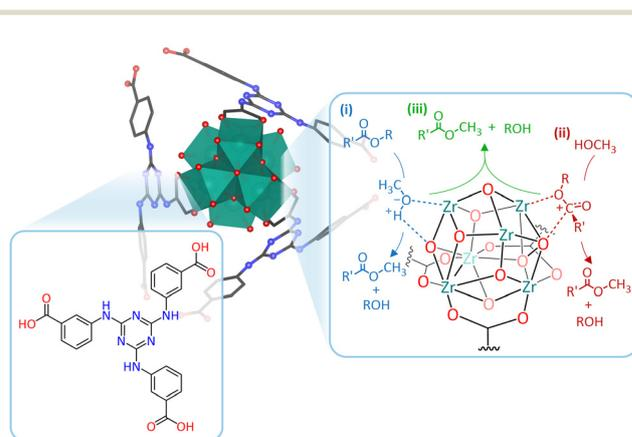
Fig. 26 Structural representation of the  $Zr_6$  cluster in TATAB(Zr) and TATAB linker along with a scheme for the three proposed reaction pathways for the transesterification of triglyceride. Adapted from ref. 317.
