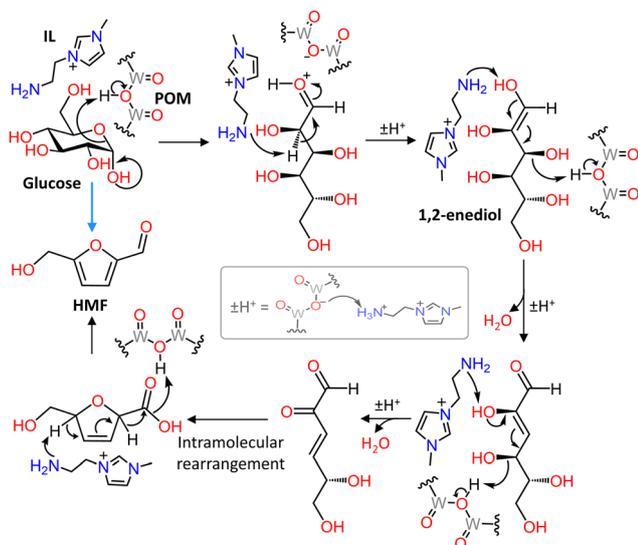
Fig. 14 Proposed mechanism for the conversion of glucose to HMF catalyzed by an HPA with an IL cation *via* formation of a 1,2-enediol intermediate that then undergoes dehydration to HMF through synergistic contributions of the IL cation and the HPA.
