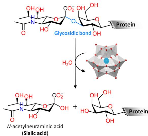
Fig. 15 Hydrolysis of the terminal glycosidic bond of an example glycan chain of a glycoprotein resulting in the release of a sialic acid catalyzed by  $\text{M}_3[\text{EA}_{12}\text{O}_{40}]^{3-}$  ( $\text{M} = \text{H}^+, \text{Na}^+, \text{K}^+$ ;  $\text{E} = \text{P}^{5+}$  or  $\text{Si}^{4+}$ ;  $\text{A} = \text{W}^{6+}$  or  $\text{Mo}^{6+}$ ).
