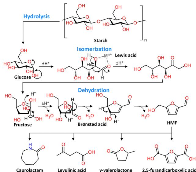
**Fig. 13** Proposed mechanism for the conversion of cellulose to HMF *via* hydrolysis to glucose, which is then isomerized to fructose (catalyzed by a Lewis acid) that in turn then undergoes dehydration to HMF (catalyzed by a Brønsted acid). Some of the value-added chemicals that can be made from HMF are also shown at the bottom.
