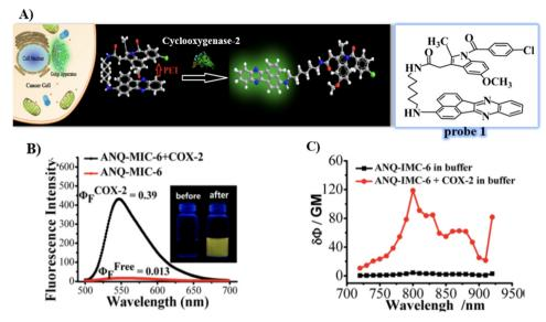
Fig. 1 (A) Detection mechanisms of probe 1 for COX-2. (B) Fluorescence emission spectra of probe 1 with and without addition of COX-2. (C) Twophoton spectra of probe 1 in the absence and presence of COX-2. Reproduced with permission from ref. 55. Copyright 2013, American Chemical Society
