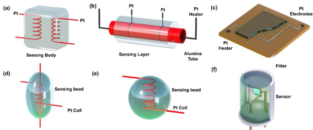
Fig. 5 Chemiresistive gas sensors are commonly built using various structures, including (a) sintered blocks, (b) thin alumina tube coatings, (c) screen-printed thick films, (d) small beads with coil and needle electrodes, (e) small beads with a single coil (heater and electrode), and (f) practical sensor elements assembled with metal caps and filters. Redraw the picture with permission from ref. 60 Copyright 2023 Elsevier.
