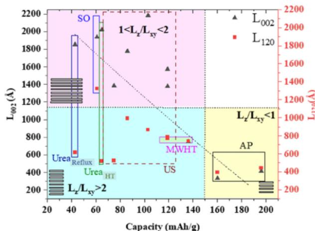
**Fig. 9** Correlation between the capacities obtained from the CV of the first cycle and structural coherence lengths  $L_z$  and  $L_{xy}$  obtained from the XRD analysis for the  $\text{Cu}_2(\text{OH})_3(\text{NO}_3)$  series of samples with US: ultra-sonification, AP: alkaline precipitation, MWHT: microwave high-temperature, and SO: salt and oxide method. Reproduced with permission from ref. 185. Copyright (2023), the American Chemical Society.
