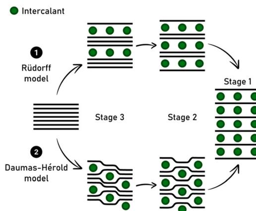
Fig. 4 Schematic representation of the Rüdorff model *versus* the Daumas-Hérold model, considering the flexible feature of graphene sheets. This model describes the continuous transformation from third to second stage GIC.
