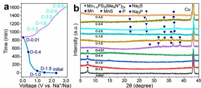
**Fig. 5** (a) Initial charge–discharge curve of the  $\text{Mn}_{1-x}\text{PS}_3(\text{Me}_4\text{N}^+)_{2x}$  electrode at  $0.05 \text{ A g}^{-1}$  and (b) corresponding *ex situ* XRD patterns at different voltage stages. Reproduced with permission from ref. 132. Copyright (2024), Elsevier.
