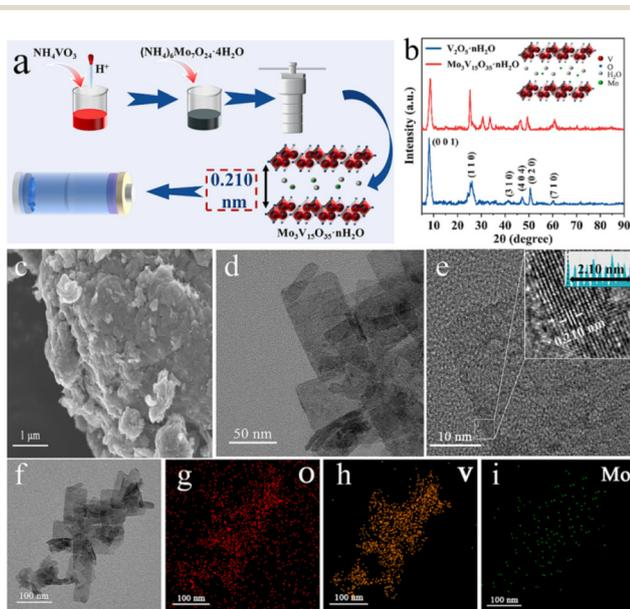
**Fig. 7** (a) Schematic of the sample preparation of  $\text{Mo}_3\text{V}_{15}\text{O}_{35}\cdot n\text{H}_2\text{O}$ . (b) XRD patterns of  $\text{V}_2\text{O}_5\cdot n\text{H}_2\text{O}$  and  $\text{Mo}_3\text{V}_{15}\text{O}_{35}\cdot n\text{H}_2\text{O}$ . (c) SEM image, d and (e) TEM and HRTEM images, and (f–i) TEM elemental mapping images of  $\text{Mo}_3\text{V}_{15}\text{O}_{35}\cdot n\text{H}_2\text{O}$ . Reproduced with permission from ref. 148. Copyright (2024), Elsevier.
