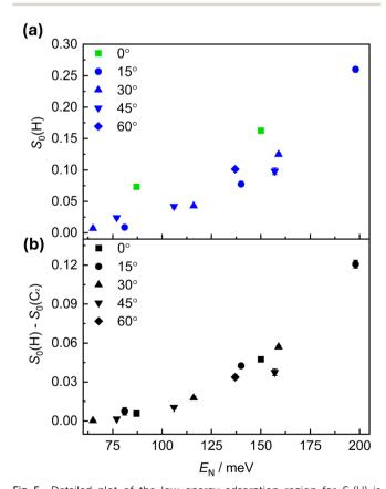
Fig. 5 Detailed plot of the low energy adsorption region for  $S_0(H)$  is shown in (a). Green symbols indicate the values for normally incident  $O_{2}$ , with blue symbols used for all other experimental  $\theta_i$ . The difference between  $S_0(H)$  and  $S_0(C)$  is shown in (b). For both graphs, the symbol shapes indicate the angle of incidence,  $\theta_{i}$ .
