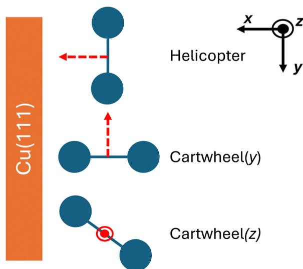
**Fig. 2** Schematic representation of the different geometries  $O_2$  can adopt when colliding with a Cu(111) surface. The red arrows indicate the rotation axes for the three geometries: helicopter (H), cartwheel- $y$  ( $C_y$ ), and cartwheel- $z$  ( $C_z$ ).
