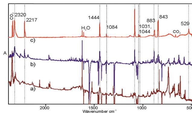
**Fig. 3** Identification of propynylphosphine **3** among the phosphabutyne **1** photolysis products in solid argon. Traces (a) and (b) are difference spectra (after-minus-before photolysis) showing the net effects of, respectively, 76 h and 3 h of Hg-lamp irradiation (concentration of **3** peaks at the beginning photolysis); trace (c) represents the spectrum of pure **3** isolated in solid Ar. Numbers give the band wavenumbers assigned to **3**.
