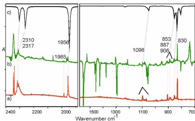
Fig. 5 Identification of propadienylphosphine (**5**) among the phosphabutyne (**1**) photolysis products in solid argon. Trace (a) represents the spectrum of an authentic (synthesized) sample of **5** isolated in solid Ar. Trace (b) is the difference spectrum (after-minus-before photolysis) showing the net effects of 76 h of Hg-lamp irradiation; traces (c) illustrate B3LYP/aug-cc-pVTZ predictions (frequency scaled by 0.96) for **3**. Numbers give the band wavenumbers assigned to **5**.
