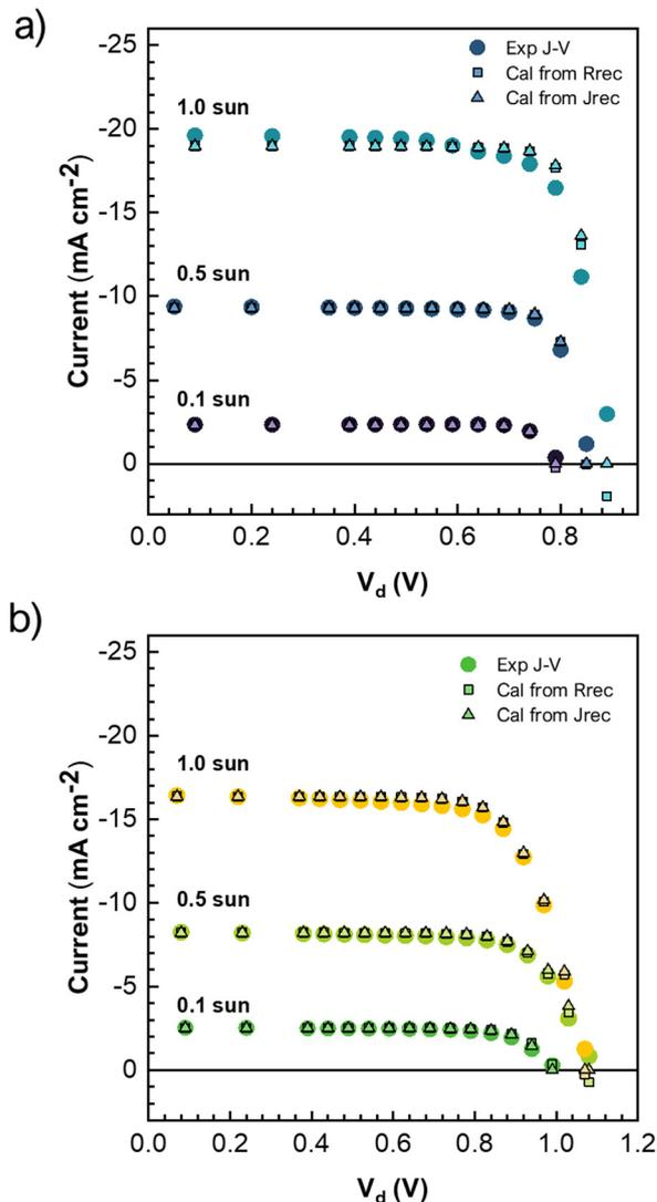
Fig. 3 Experimental  $j$ - $V$  curve (dots) and its reconstruction (eqn (4)) by using  $m$ -values obtained either the slope of  $R_{\text{rec}}$  vs.  $V_{\text{app}}$  (squares) or from  $J_{\text{rec}}$  (eqn (2), triangles) at different illumination intensities for (a) PEDOT:PSS/ $C_{60}$  and (b) MeO-2PACz/ $C_{60}$  devices. The voltage applied is optimized by the series resistance contribution as  $V_d = V_{\text{app}} - jR_s$ .
