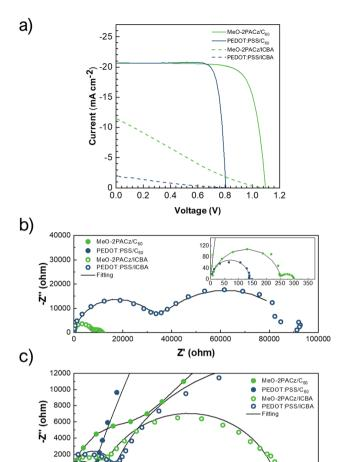
Fig. 1 (a) j-V curves of devices with different selective contacts at 1 sun illumination. Nyquist plots of the devices measured at  $V_{oc}$  (b) and  $j_{sc}$  (c) conditions under 0.1 sun illumination. The inset in (b) shows a zoomed-in Nyquist plot for the devices with C<sub>60</sub>.
