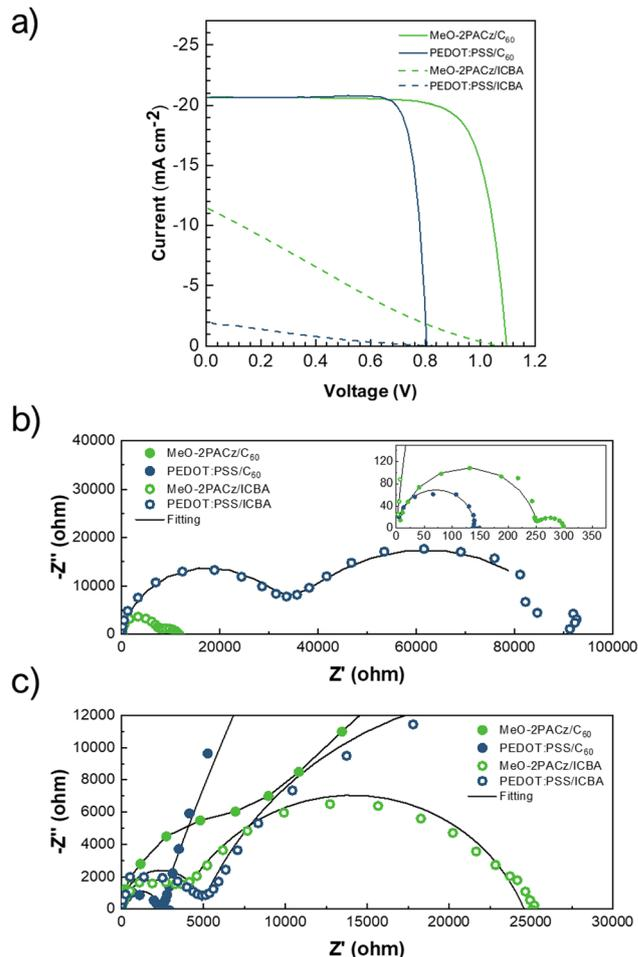
Fig. 1 (a)  $j$ - $V$  curves of devices with different selective contacts at 1 sun illumination. Nyquist plots of the devices measured at  $V_{oc}$  (b) and  $J_{sc}$  (c) conditions under 0.1 sun illumination. The inset in (b) shows a zoomed-in Nyquist plot for the devices with  $C_{60}$ .
