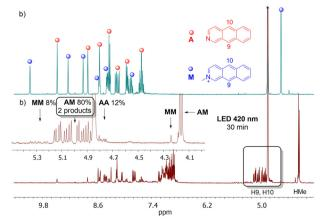
Fig. 4  $^{1}$ H NMR spectrum of the mixture of *N*-methyl-2-azaanthracene (**M**) iodide and azaanthracene (**A**) before (a) and after (b) 30 min of irradiation at 365 nm (left) and 420 nm (right) measured in methanol- $d_4$  at 298 K at 300 MHz. The inserts show the aliphatic regions of the spectra. Region 5.4–4.7 ppm is characteristic for H9 and H10 protons of dimers: 5.4–5.2 ppm for **MM**, 5.2–4.9 ppm for **AM**, 4.9–4.7 ppm for **A**.
