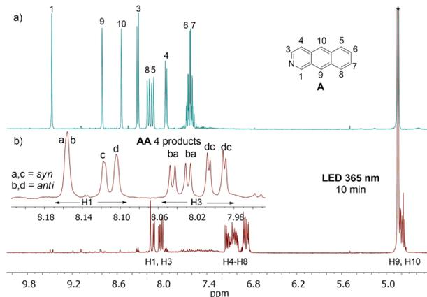
Fig. 2  $^1\text{H}$  NMR spectrum of 2-azaanthracene (**A**) (a) and the photoproduct after 10 min of irradiation at 365 nm (mixture of **AA** isomers) (b) measured in methanol- $d_4$  at 298 K at 300 MHz. The insert shows the region of the spectrum above 7.95 ppm with signals of protons H1 (singlets) and H3 (doublets) - near the nitrogen atom. The initial concentration of **A** was  $4.7 \times 10^{-3}$  M.
