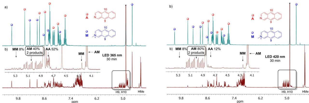
Fig. 4  $^1\text{H}$  NMR spectrum of the mixture of *N*-methyl-2-azaanthracene (**M**) iodide and azaanthracene (**A**) before (a) and after (b) 30 min of irradiation at 365 nm (left) and 420 nm (right) measured in methanol- $d_4$  at 298 K at 300 MHz. The inserts show the aliphatic regions of the spectra. Region 5.4–4.7 ppm is characteristic for H9 and H10 protons of dimers: 5.4–5.2 ppm for **MM**, 5.2–4.9 ppm for **AM**, 4.9–4.7 ppm for **A**.
