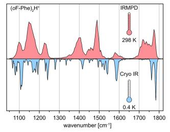
Fig. 2 Comparison of experimental IR spectra of the protonated orthofluorophenylalanine dimer (oF-Phe)<sub>2</sub>H<sup>+</sup> generated by room-temperature IRMPD spectroscopy (red) and cryogenic IR spectroscopy in helium droplets (0.4 K, blue).
