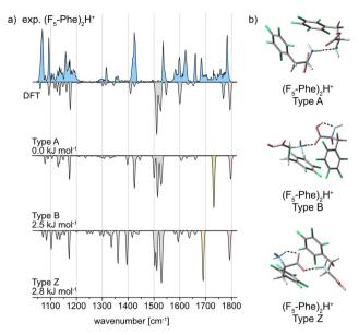
Fig. 4 (a) Infrared spectra of the proton-bound homodimer of pentafluorophenylalanine. The experimental IR spectrum is depicted as a light blue trace. Computed spectra of the low-energy structures are shown as gray inverted traces with distinct absorption bands highlighted according to the vibration they originate from. Relative free energies at 90 K are indicated. (b) Global minimum structures of the A, B, and Z type interactions for (F<sub>5</sub>-Phe)<sub>2</sub>H<sup>+</sup>
