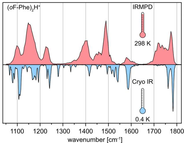
Fig. 2 Comparison of experimental IR spectra of the protonated *ortho*-fluorophenylalanine dimer  $(oF\text{-Phe})_2\text{H}^+$  generated by room-temperature IRMPD spectroscopy (red) and cryogenic IR spectroscopy in helium droplets (0.4 K, blue).
