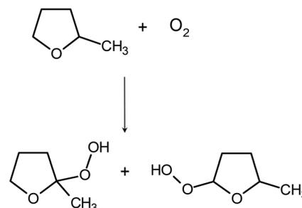
**Scheme 1** Oxidation of 2-methyltetrahydrofuran. Two isomers of 2-methyltetrahydrofuran hydroperoxide are formed: 2-methyl-2-peroxytetrahydrofuran (left) and 2-methyl-5-peroxytetrahydrofuran (right).
