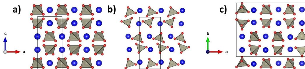
Fig. 1 Crystal structures of the scheelite-type oxides for (a) tetragonal  $I4_1/a$ , (b) orthorhombic  $Pnma$ , and (c) monoclinic  $P2_1/c$ . Note that the monoclinic  $P2_1/c$  unit cell has been tripled along the  $a$  axis.
