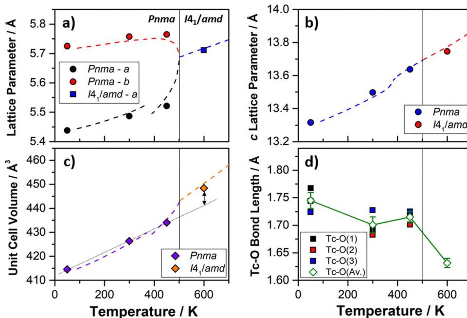
Fig. 3 Temperature dependence of the (a) and (b) lattice parameters, (c) unit cell volume, and (d) the Tc–O bond distances for  $\text{TiTcO}_4$  derived from the Rietveld refinements of the neutron powder diffraction data. Where not shown, the error bars are smaller than the symbols. The dashed lines in (a)–(c) are the results from the previous synchrotron X-ray diffraction study.<sup>33</sup> The dotted line in (c) drawn to guide the eyes.
