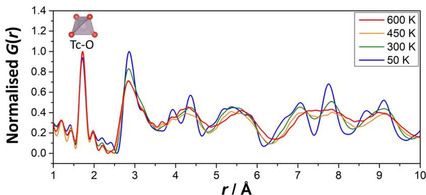
Fig. 4 Variable temperature neutron pair distribution function data of  $\text{TiTcO}_4$  at 50 (blue), 300 (green), 450 (orange), and 600 K (red).
