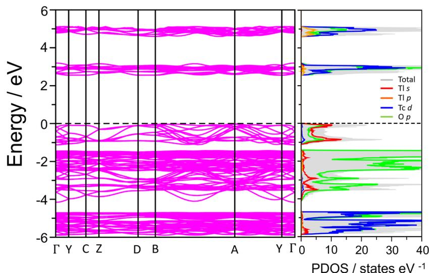
Fig. 6 Electronic band structure and partial density of states (PDOS) of  $\text{TlTcO}_4$  in the monoclinic  $P2_1/c$  structure calculated using the Tran–Blaha modified Becke–Johnson (TB-mBJ) potential, showing a bandgap of 2.53 eV.
