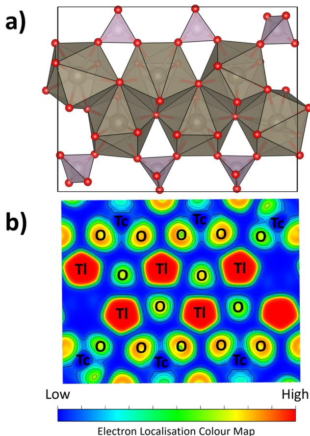
Fig. 7 (a) Structural model of  $\text{TlTcO}_4$  in the monoclinic  $P2_1/c$  space group, fit from the 50 K POWGEN neutron pair distribution function data. (b) Iso-surface maps illustrating bonding interactions through the electron localisation function (ELF) in the  $\langle 001 \rangle$  plane generated for the geometry-optimised structure of  $\text{TlTcO}_4$  in the monoclinic  $P2_1/c$  space group.
