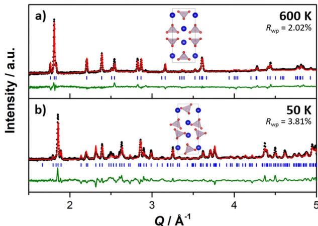
Fig. 2 Rietveld refinements to the neutron Bragg data of TlTcO<sub>4</sub>, collected on the POWGEN diffractometer at (a) 600 K refined to the tetragonal *I*<sub>41</sub>/*amd* space group, and (b) 50 K refined to the orthorhombic *Pnma* space group. The black circles represent the data, the red line represents the fit to the data, the green line represents the difference between the data and the fit, and the blue dashes represent the space group-allowed reflections.
