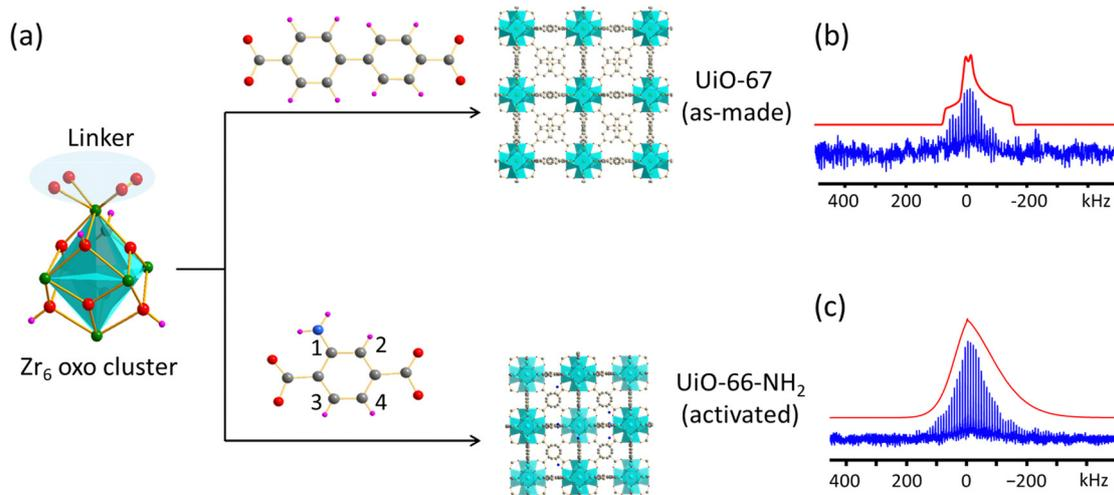
Fig. 3 The short- and long-range structure of UiO-67 and UiO-66-NH<sub>2</sub> are shown in (a), along with their respective organic linkers. The experimental (blue) and simulated (red) static <sup>91</sup>Zr NMR spectra of UiO-67 and UiO-66-NH<sub>2</sub> at 35.2 T are given in (b) and (c), respectively.
