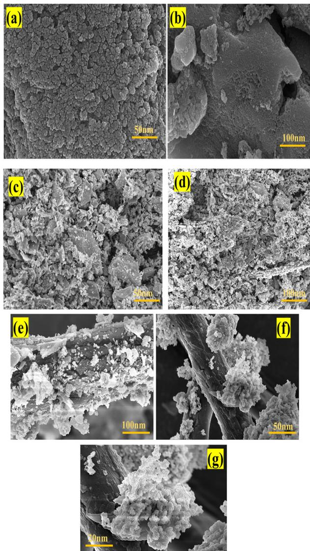
Fig. 6 FESEM images of  $g\text{-C}_3\text{N}_4$  (a), (b), MgO NPs (c), (d) and MgCN nanocomposites (e)–(g) at different magnifications.
