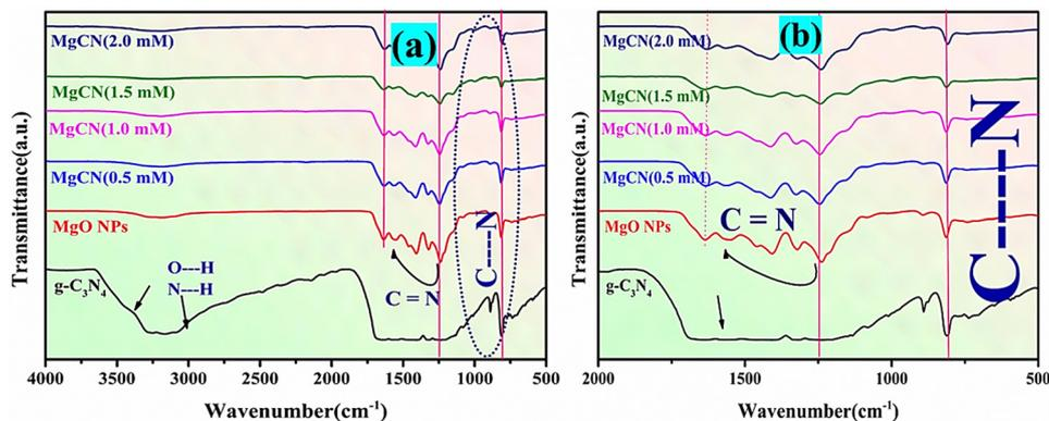
Fig. 5 FTIR spectra of (a) g-C<sub>3</sub>N<sub>4</sub>, MgO NPs, and MgCN nanocomposites, and (b) inset view of the MgCN bonding structure.
