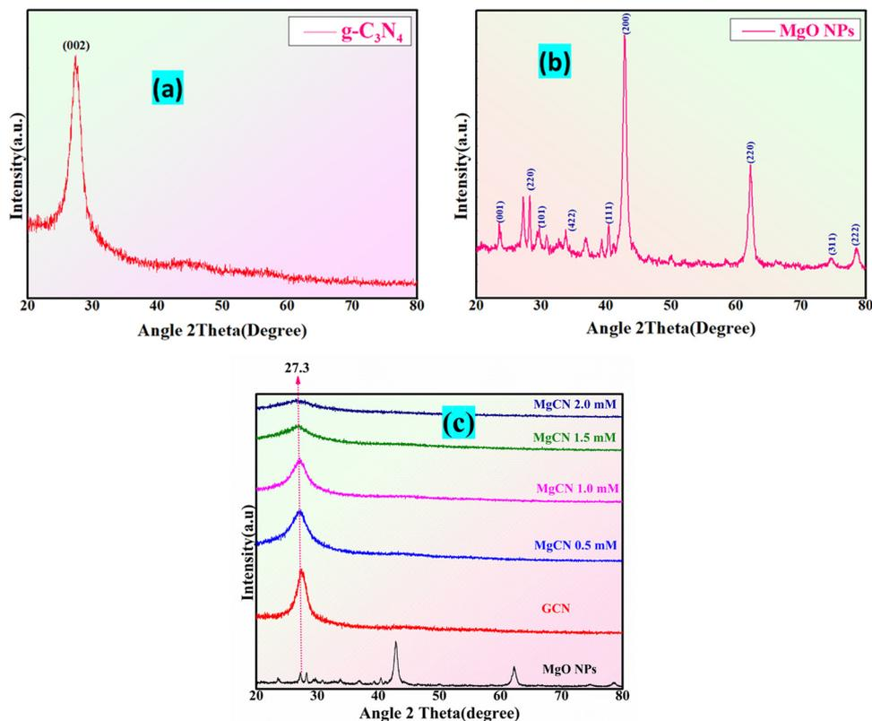
Fig. 4 XRD pattern of (a) g-C<sub>3</sub>N<sub>4</sub>, (b) MgO NPs, and (c) MgCN composites at varied conc. (0.5, 1.0, 1.5 and 2.0 mM).
