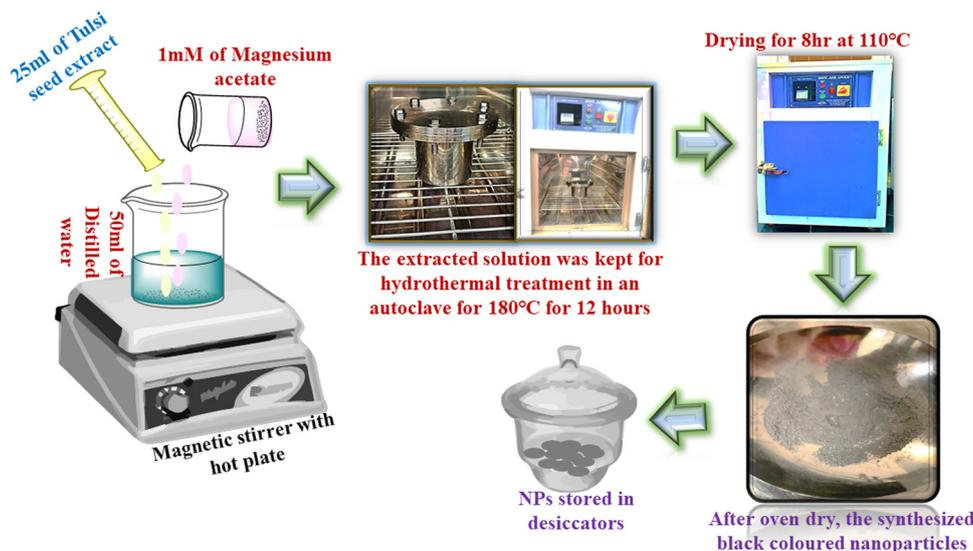
Fig. 2 Synthesis of MgO NPs using TSE.
