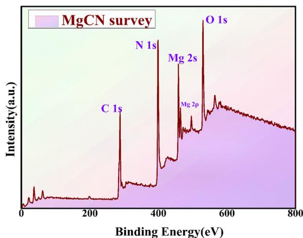
Fig. 10 XPS survey spectra for the MgCN nanocomposite.
