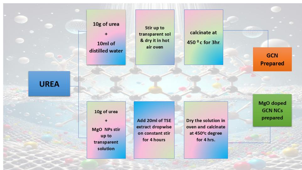
Fig. 3 Fabrication of MgO doped g-C<sub>3</sub>N<sub>4</sub> nanocomposites (MgCN) at varying conc.
