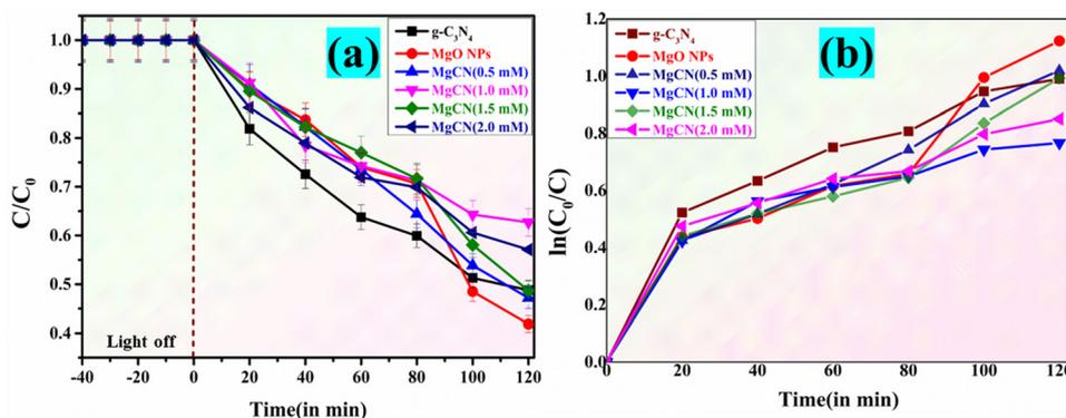
Fig. 12 (a)  $C/C_0$  Comparison of the degradation of Methylene Blue dye (dark and light mode); (b)  $\ln C_0/C_t$  as a function of visible light irradiation period with MgO,  $g-C_3N_4$  and MgCN nanocomposites.
