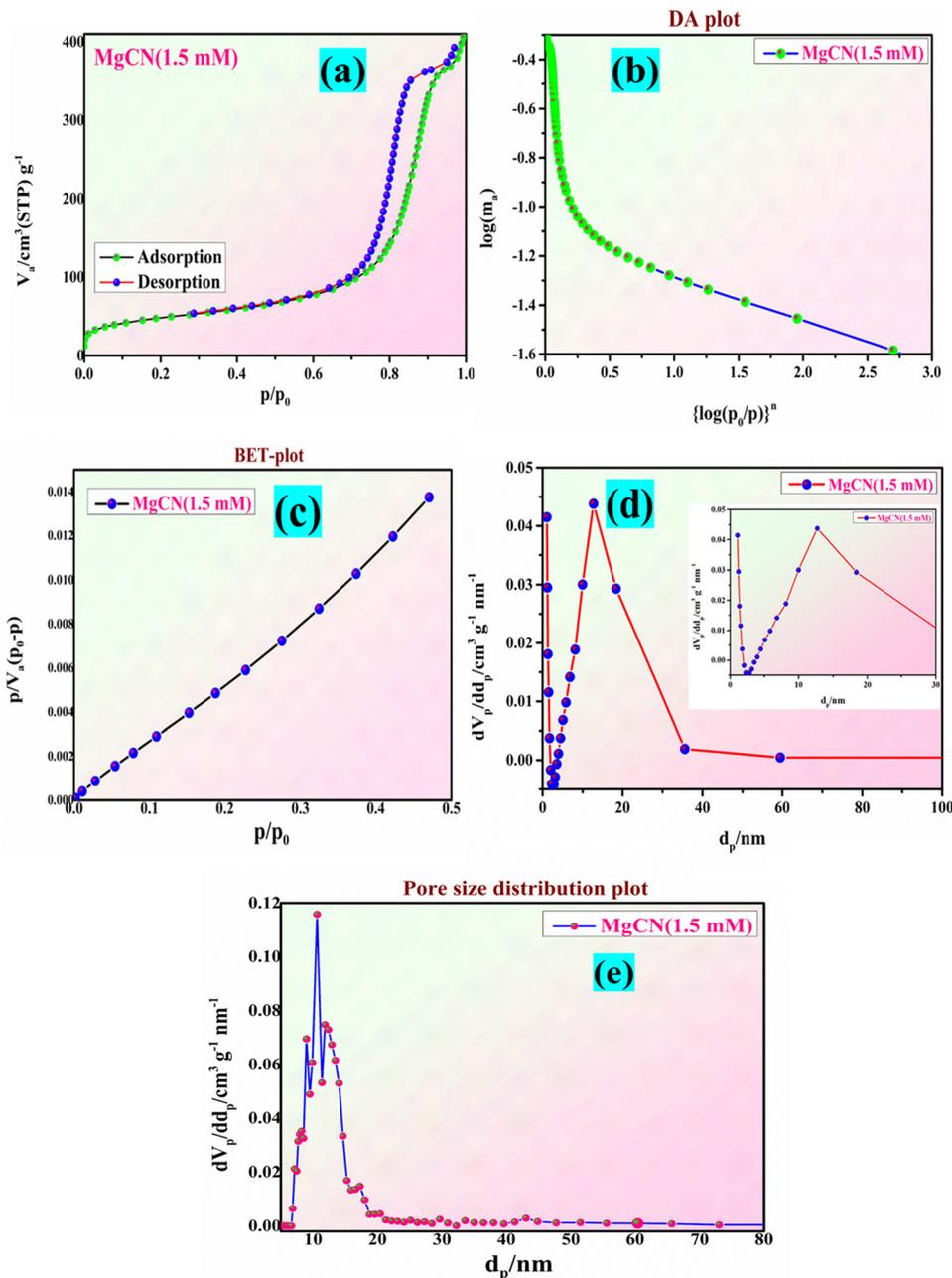
Fig. 9 The adsorption–desorption adsorption–surface area curve of the (a) and (b) MgO/g-C<sub>3</sub>N<sub>4</sub> nanocomposite (MgCN), together with the BET and BJH plot (c) and (d) (inset view) and the pore distribution curve (e).
