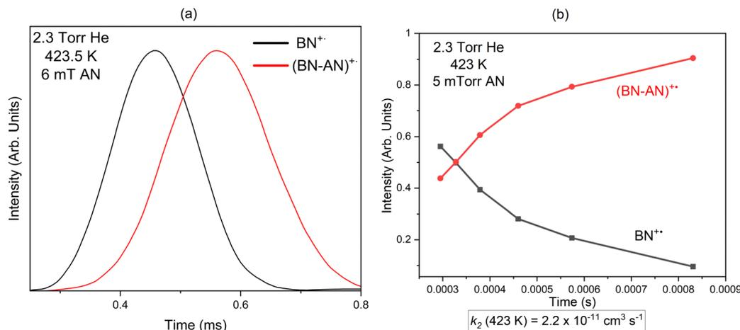
Fig. 2 (a) Arrival time distribution (ATDs) and (b) time profiles of the reactant and product ions for the reaction of the benzonitrile radical cation ( $\text{BN}^{+\bullet}$ , black line) with acrylonitrile (AN) resulting in the formation of the adduct  $(\text{BN-AN})^{+\bullet}$ , red line.
