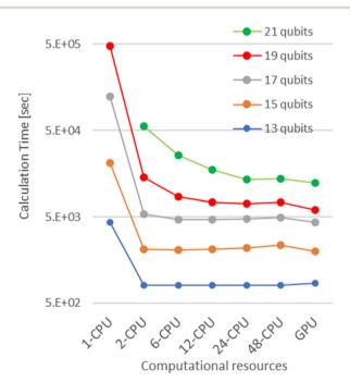
Fig. 3 The comparison of the calculation time of numerical simulations with multi-CPUs or a single-GPGPU
