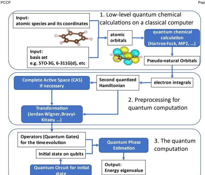
Fig. 1 The workflow of our quantum chemical calculation on a quantum computer. It consists of three parts. (1) Low-level quantum chemical calculations on a classical computer, which aims to obtain the information of molecular orbitals. (2) Pre-processing for quantum computation, which is to transform the above obtained molecular orbitals into quantum gates and gubits. (3) The guantum computations (using the simulator, or if possible, using a quantum computer)
