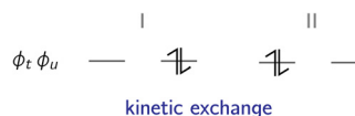
Fig. 2 The kinetic exchange effect stems from the interaction of the ionic forms (I and II) within the active space with the reference determinants ( i.e. the neutral forms within the active space).
