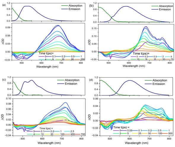
Fig. 8 Transient absorption spectra plotted as a function of different delays after the pump pulse for (a) 2 and (b) 3 in EtOH, and (c) 2, and (d) 3 in THF at T = 298 K. Steady-state absorption and emission spectra are shown for comparison of GSB and SE.
