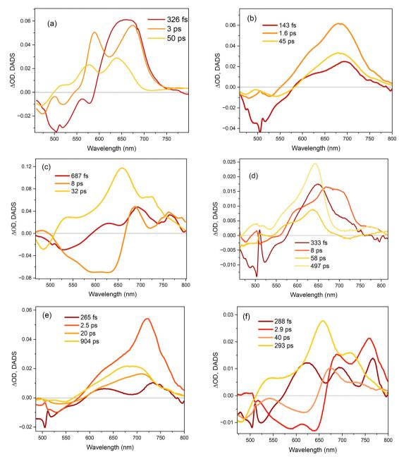
Fig. 9 Decay associated difference spectra (DADS) for (a) 1, (b) 2 and (c) 3 in ethanol, and (d) 1, (e) 2 and (f) 3 in THF. The DADS were obtained from global fits of the kinetic traces to the transient absorption spectra.
