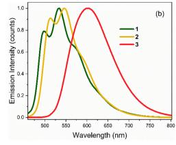
Fig. 3 Steady-state emission spectra of 1-3 at T = 298 K in: (a) EtOH, and (b) THF. Spectra are normalised to reflect relative quantum yields (in THF, all three chromophores have similar quantum yields).
