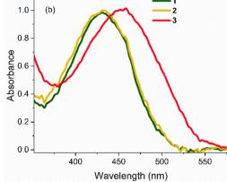
Fig. 2 Steady-state absorption spectra of 1-3 at T = 298 K in: (a) EtOH, and (b) THF. In both solvents, the spectra for 1 and 2 are nearly identical. All spectra are normalised to unit intensity
