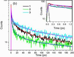
Fig. 6 Ultrafast fluorescence up-conversion of 1-3 excited at ≈ 400 nm in (a) EtOH and (b) THF. Time-resolved emission decays were recorded at the wavelength maximum of the respective emission spectrum at T = 298 K. The emission counts are presented on a log scale after background subtraction to emphasise the multi-exponential nature of the decays. Insets show a magnified view of the sub-picosecond decay and rising components. The grey curve in the insets show the instrument response function
