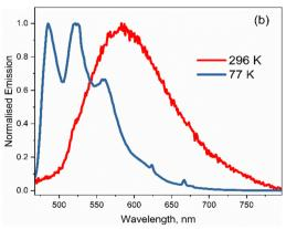
Fig. 5 (a) Emission spectra for 3 in EtOH as a function of temperature. The inset highlights the initial red shift in the emission maximum on decreasing from T = 296 K to 180 K. (b) Normalised emission spectra at room temperature and at T = 77 K showing the emergence of vibronic structure at low temperature
