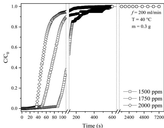
**Fig. 6** SO<sub>2</sub> breakthrough curves of KCC-1/DES1 at different SO<sub>2</sub> concentrations.
