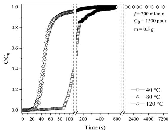
Fig. 8 SO<sub>2</sub> breakthrough curves of KCC-1/DES1 at different temperatures.
