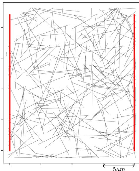
Fig. 1 Computationally generated nanowire network geometry with a density of 0.67 nanowires per  $\mu\text{m}^2$ . The black lines represent the coated metal nanowires (in our case simulated to be Ag/PVP core-shell nanowires). The red vertical lines represent the metallic leads acting as electrodes. The scale bar at the bottom right part of the plot indicates 5  $\mu\text{m}$  in length.
