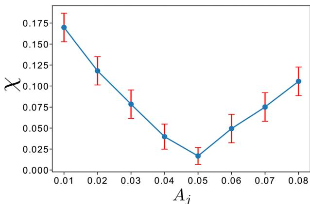
Fig. 9 Fixing  $\alpha_j = 1.1$  in Fig. 8, one can visualize the misfit function (average) plotted in terms of  $A_j$ ; the minimum is located at  $A_{\text{min}} = 0.05$ , corresponding to the original prefactor set in the target NWN system. The average of  $\chi$  was computed for  $N_{\text{tg}} = 60$  different target NWNs with an accuracy of 95% and standard deviations shown as error bars.
