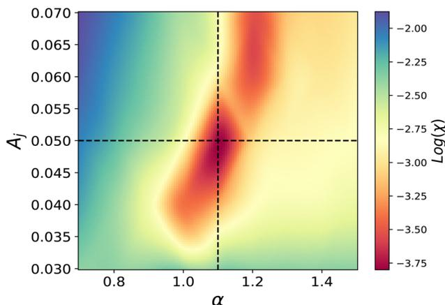
Fig. 8 Surface contour plot of the (logarithm) misfit function in terms of  $\alpha \equiv \alpha_j$  and  $A_j$  taken for a NWN with  $N_j = 900$ . The crossing of the horizontal and vertical dashed lines indicates the minimum of the  $\log(\chi)$  surface, matching the parameters initially set for the target NWN system which were  $\alpha_j = 1.1$  and  $A_j = 0.05$ .
