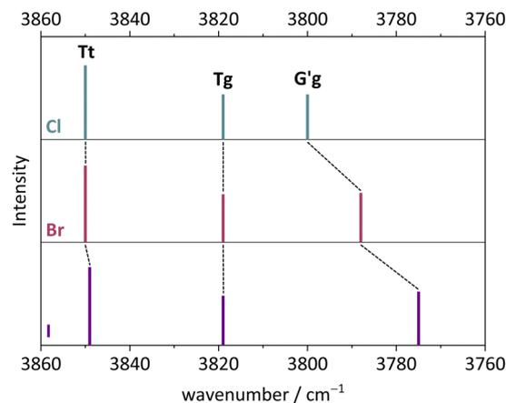
Fig. 8 Comparison between the calculated harmonic wavenumbers and IR intensities for the monomer conformers of Cl, Br, I, calculated at B3LYP-D3(BJ)/def2-QZVP level.
