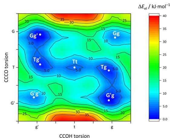
Fig. 3 Contour plot of the two dimensional orca relaxed full cycle scan of the CCCO angle and the CCOH angle of the Cl monomer at B97-3c level with a stepsize of  $20^\circ$ . The shown electronic energy difference is referred to the structure with the lowest calculated energy ( $Gg'$ , respectively  $G'g$  conformer).
