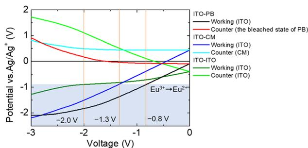
Fig. 4 Electrode potential measurements using the two-electrode devices of the  $\text{Eu}(\text{hfa})_3(\text{H}_2\text{O})_2$  solution: (ITO–PB (ITO as the WE: the black line and the bleached state of PB as the CE: the red line), ITO–CM (ITO as the WE: the blue line and CM as the CE: the light blue line), ITO–ITO (ITO as the WE: the deep green line and ITO as the CE: the green line).
