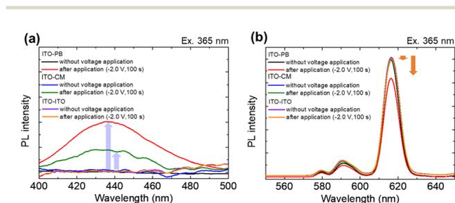
Fig. 8 Emission spectra of the Eu complex in the two-electrode devices (ITO–PB, ITO–CM, and ITO–ITO device) before and after applying a reduction voltage of  $-2.0$  V for 100 s at approximately (a) 430 nm and (b) 615 nm. The excitation wavelength was 365 nm.
