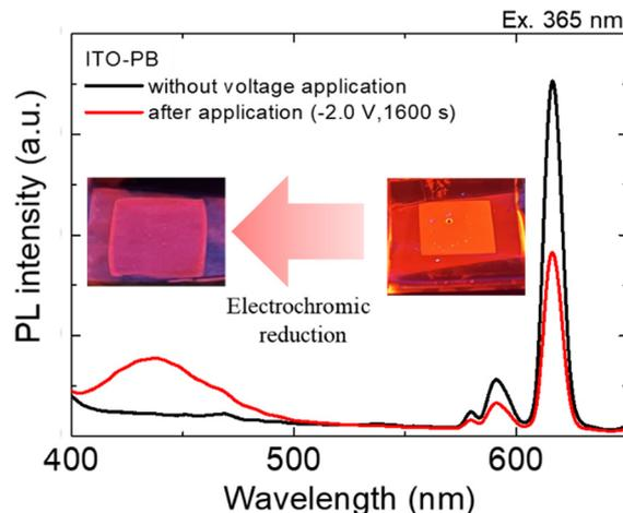
Fig. 6 Emission spectra of the  $\text{Eu}(\text{hfa})_3(\text{H}_2\text{O})_2$  solution in  $\text{PEG}_{400}$  using the ITO–PB device before and after the application of reducing voltages. The excitation wavelength was 365 nm.
