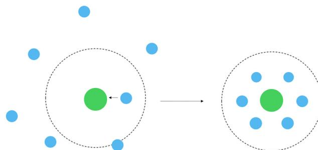
**Fig. 7** Schematic depiction of the transition between the MgHe dimer model system to an explicit solvation model for large densities. The collision cross section is shown as dotted circle (Mg: green, He: blue).
