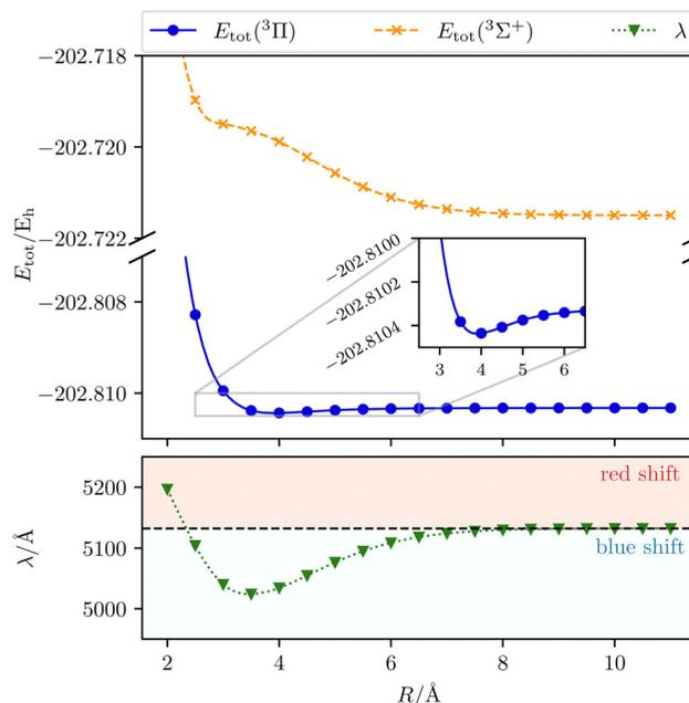
Fig. 3 The transition wavelength  $\lambda$  ( $^3\Pi \rightarrow ^3\Sigma^+$ ) as well as the total initial-state energy  $E_{\text{tot}}$  as a function of the Mg–He distance  $R$ . Calculated with CD-CCSD ( $\delta = 5$ ) using the unc-aug-cc-pCVQZ basis for Mg and the unc-aug-cc-pVDZ basis for He.
