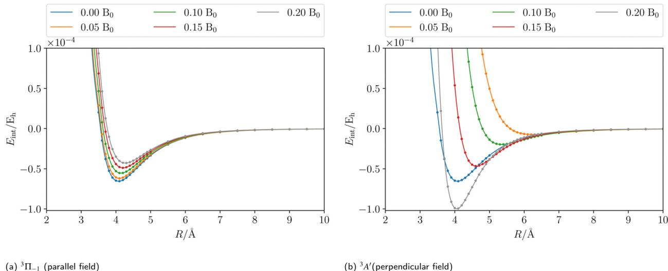
Fig. 4 The counterpoise corrected<sup>185,186</sup> CCSD interaction energy of the initial state of the MgHe triplet dimer plotted as a function of the external magnetic field strength in a parallel (a) and perpendicular (b) orientation, respectively. The calculations were performed using the unc-aug-cc-pCVQZ basis for Mg and an unc-aug-cc-pVDZ basis for He.
