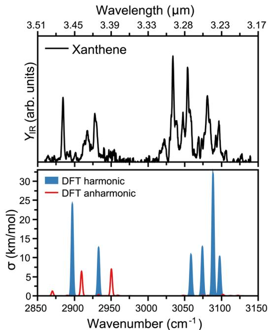
Fig. 2 Top: Infrared spectrum of neutral xanthene recorded in the  $2850$  to  $3150 \text{ cm}^{-1}$  range, using an infrared OPO/OPA laser. The top axis presents the corresponding range in wavelength. Bottom: DFT calculated vibrational spectrum of xanthene, with harmonic computations in blue and combination bands and overtones in red. For visualization purposes, Gaussian functions are built around each vibration, with a FWHM of  $2 \text{ cm}^{-1}$ .
