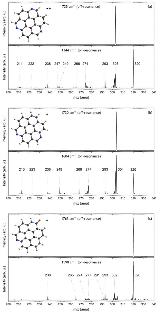
Fig. 2 Mass spectra of isolated  $TAC^+$  (a),  $TACH^+$  (b) and  $[TAC-H + H_2O]^+$  (c) after exposure to off-resonance (top panel) and on-resonance (bottom panel) infrared radiation. The wavenumber of the IR radiation is depicted in each respective panel. The proposed geometry for the  $[TAC-H + H_2O]^+$  species is discussed in Section 3.4.
