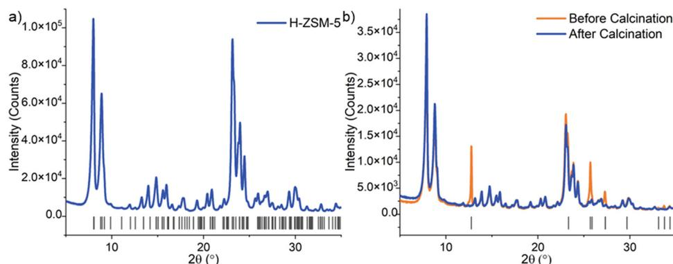
Fig. 1 PXRD patterns of zeolite precursors H-ZSM-5 with indexing lines of the references ZSM-5 structures (a) and Mo4-Z5 before (blue line) and after (orange line) calcination with indexing lines of the crystalline MoO<sub>3</sub> phase are shown below the patterns (b).
