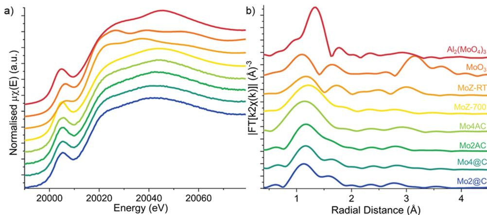
Fig. 9 Mo K-edge XANES spectra (a) and  $k^2$  weighted FT-EXAFS magnitude (b) of Mo2-Z5-@C, Mo4-Z5-@C, Mo2-Z5-AC, and Mo4-Z5-AC sample, and MoZ-700, MoZ-RT, MoO<sub>3</sub>, and Al<sub>2</sub>(MoO<sub>4</sub>)<sub>3</sub> reference (from bottom to top).
