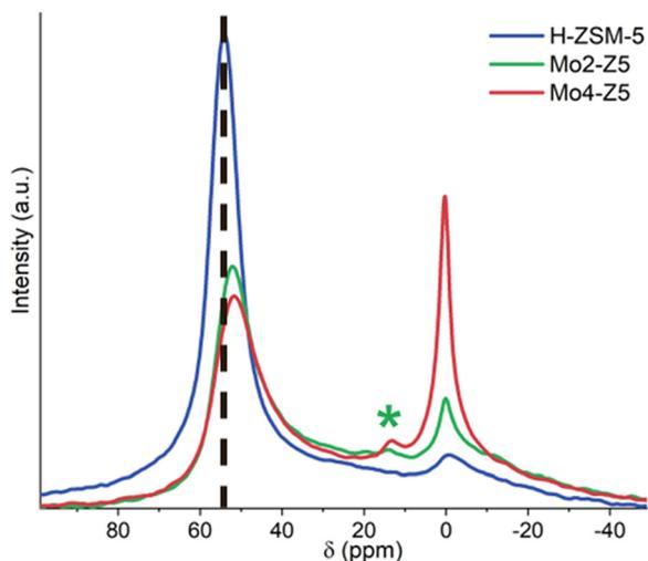
Fig. 2 <sup>27</sup>Al MAS-NMR spectra of H-ZSM-5, Mo2-Z5 and Mo4-Z5 (the \* indicates the location of the chemical shift for  $\text{Al}_2(\text{MoO}_4)_3$  at 14 ppm).
