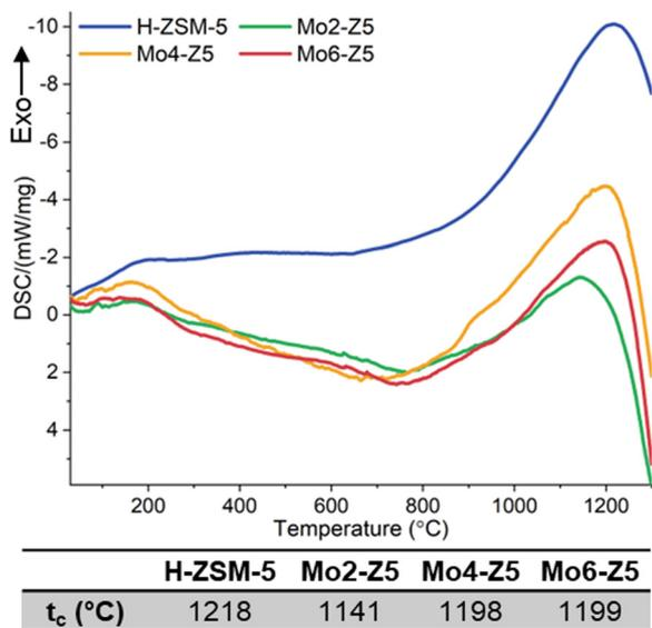
Fig. 4 DSC traces of H-ZSM-5, Mo2-Z5, Mo4-Z5, and Mo6-Z5.  $t_c$ s of the Mo exchanged H-ZSM-5 samples and H-form precursor are listed in Table 1. Note the weak shoulders at  $900\text{ }^\circ\text{C}$  in the Mo4-Z5 and Mo6-Z5 samples are probably due to Mo volatilisation.
