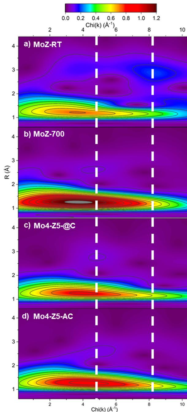
Fig. 10  $k^2$  weighted Morlet WT-EXAFS contour plot of (a) MoZ-RT, (b) MoZ-700, (c) Mo4-Z5-@C, and (d) Mo4-Z5-AC. The white dotted lines mark the  $k$ -space position of the Mo–Al/Si and Mo–Mo single scattering path at  $4.8 \text{ \AA}^{-1}$  and  $8.3 \text{ \AA}^{-1}$ . All four contours are plotted to the same color scale.
