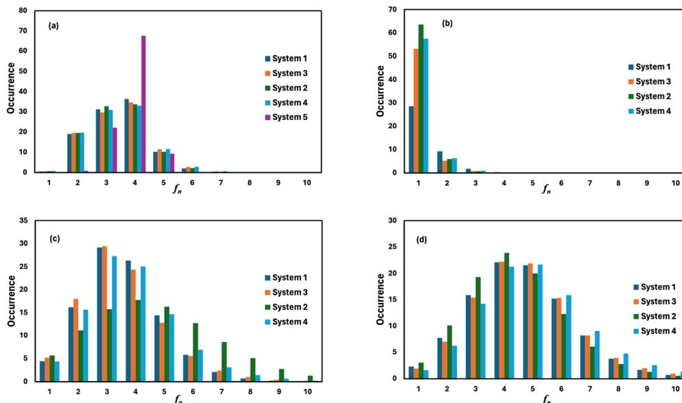
Fig. 7 The fraction of water molecules forming ' $n$ ' number of hydrogen bonds of (a)  $\text{H}_2\text{O}\cdots\text{H}_2\text{O}$ , (b)  $\text{H}_3\text{O}^+\cdots\text{H}_2\text{O}$ , (c)  $\text{HSO}_4^-\cdots\text{H}_2\text{O}$ , and (d)  $\text{SO}_4^{2-}\cdots\text{H}_2\text{O}$  type in the presence of  $\text{VOSO}_4$ .
