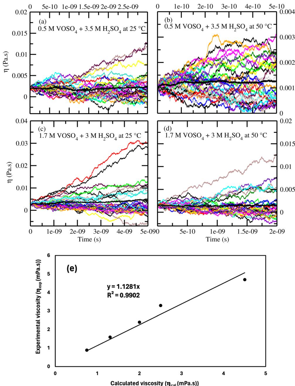
Fig. 10 (a)–(d) The computed viscosity for systems 1–4. (e) The correlation between the calculated and experimental<sup>31</sup> viscosity.
