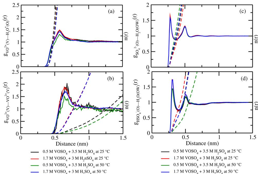
Fig. 5 The radial distribution function for (a) vanadium of the  $\text{VO}^{2+}$  ion and oxygen of the  $\text{H}_3\text{O}^+$  ion, (b) vanadium of the two  $\text{VO}^{2+}$  ions, (c) oxygen of  $\text{SO}_4^{2-}$  and oxygen of the  $\text{H}_2\text{O}$  molecule and, (d) oxygen of  $\text{HSO}_4^-$  and oxygen of the  $\text{H}_2\text{O}$  interaction for systems 1–4.
