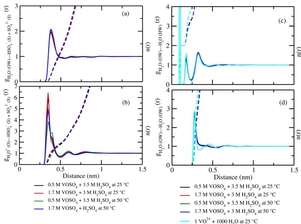
Fig. 6 The radial distribution function for (a) oxygen of  $\text{H}_2\text{O}$  and sulfur of  $\text{HSO}_4^- + \text{SO}_4^{2-}$  ion, (b) oxygen of  $\text{H}_3\text{O}^+$  and sulfur of  $\text{HSO}_4^- + \text{SO}_4^{2-}$  ion, (c) oxygen of  $\text{H}_2\text{O}$  and hydrogen of the  $\text{H}_2\text{O}$  molecule, and (d) oxygen of  $\text{H}_2\text{O}$  and oxygen of the  $\text{H}_2\text{O}$  interaction for systems 1–4.
