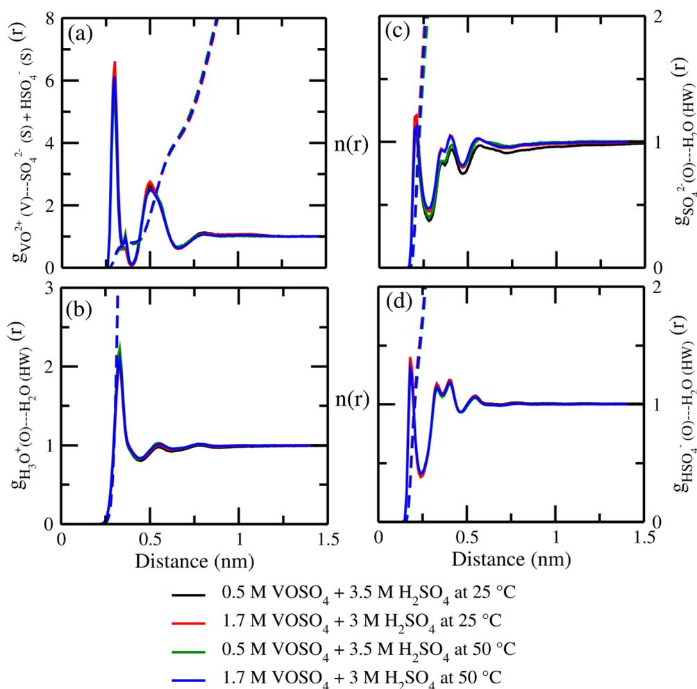
Fig. 4 The radial distribution function for (a) vanadium of the  $\text{VO}^{2+}$  ion and sulfur of the  $\text{HSO}_4^- + \text{SO}_4^{2-}$  ion, (b) oxygen of  $\text{H}_3\text{O}^+$  and hydrogen of the  $\text{H}_2\text{O}$  molecule, (c) sulfur of the  $\text{SO}_4^{2-}$  ion and hydrogen of the  $\text{H}_2\text{O}$  molecule, and (d) sulfur of the  $\text{HSO}_4^-$  ion and hydrogen of the  $\text{H}_2\text{O}$  molecule for systems 1–4.
