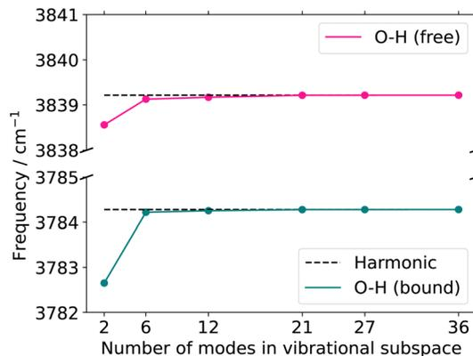
**Fig. 8** Quasi-harmonic frequencies for the two OH-stretching vibrations with increasing vibrational subspace size (B2PLYP-D3/aug-cc-pVTZ). O–H (bound) refers to the hydrogen-bonded stretching vibration of O3–H1, whereas O–H (free) refers to the hydrogen-bond-accepting stretching vibration of O4–H2. The atoms considered in each vibrational subspace are listed in the ESI<sup>†</sup> in the Table SIV. The dotted line represents the harmonic frequency at normal modes.
