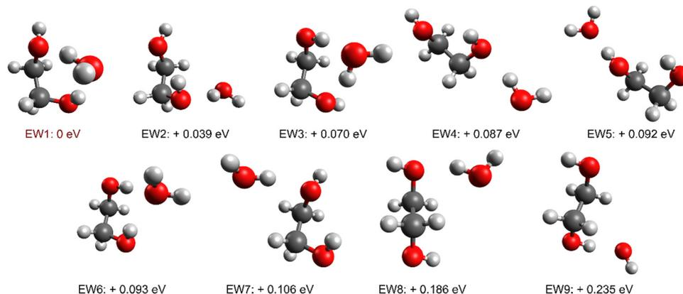
Fig. 4 All nine minimum energy structures calculated for the EG(H<sub>2</sub>O) dimer with energies given relative to the minimum energy structure, EW1.
