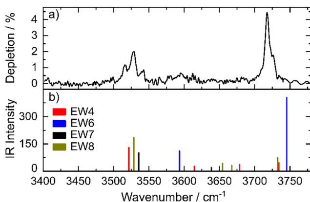
**Fig. 3** (a) The IR spectrum in the OH stretching region from an  $EG/H_2O$  mixture in helium nanodroplets. (b) Anharmonic IR spectra calculated for the conformers EW4, 6, 7, and 8 shown in Fig. 4. For the calculated spectra the intensities were weighted at ratios of 1.2/5/1/1.5 for EW4/EW6/EW7/EW8, in order to give the best agreement with experiment.
