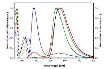
Fig. 2 The absorption (dashed line) and emission (solid line) spectra of 1 (blue), 2 (red), 3 (black), and 4 (green) in cyclohexane at 295 K. The excitation wavelengths are at the lowest-lying absorption band.
