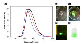
**Fig. 4** (a) Emission spectra of compound **4**, showcasing photoluminescence in cyclohexane ( $1\times10^{-5}$  M, red line) and in powder form (blue line), as well as TL in crystal form (black line). (b) Compound **4** under ambient light and (c) under UV irradiation at 365 nm. (d) TL image of the compound **4** crystal ground in a sample vial using a spatula. (e) Schematic diagram of TL corresponding to (d).
