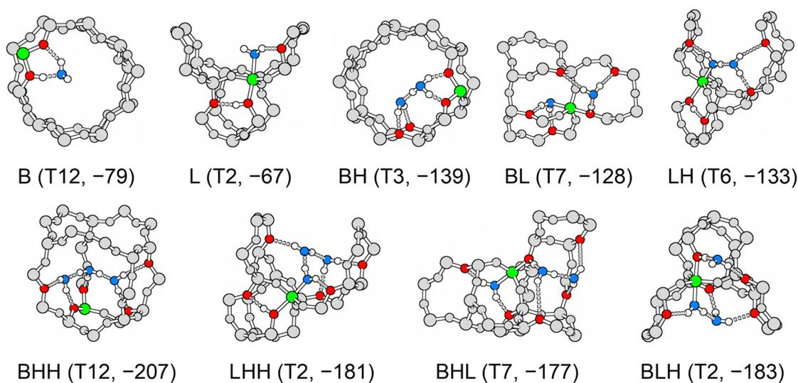
**Fig. 9** Most stable adsorption structures for each interaction motif. Framework position and MP2+ $\Delta$ CC adsorption energies in  $\text{kJ mol}^{-1}$  in parenthesis. Colour code: aluminium – green, framework oxygen accepting hydrogen bond – red, oxygen in water molecules – blue, framework silicon and oxygen – grey, hydrogen – white.
