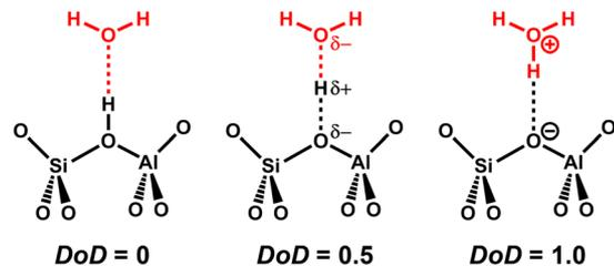
Fig. 7 Schematic representation of borderline cases of the degree of deprotonation (DoD) of the BAS, see eqn (1).
