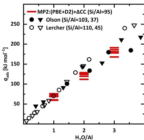
**Fig. 12** Experimental integral heats of adsorption ( $q_{\text{ads}}$ ) as reported by Liu, Lercher and co-workers<sup>3</sup> (calorimetry, empty symbols) as well as Olson, Haag, and Borghard<sup>38</sup> (isotherms, full symbols). For both, two samples with different Si/Al ratio are included. MP2+ $\Delta\text{CC}$  adsorption enthalpies (absolute values) for all six framework positions (red bars). The respective most stable adsorption motif is chosen, see Table 4.
