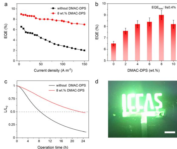
Fig. 4 (a) EQE–current density characteristics of LECs with 8 wt% and without DMAC-DPS. (b) EQE values measured at 100  $\text{cd m}^{-2}$  and different sensitizer concentrations. (c) Normalized luminance as a function of operational time with an initial of  $L_0 = 100 \text{ cd m}^{-2}$  at constant current with 8 wt% and without DMAC-DPS. (d) Image of TSF-LECs with a pattern of the abbreviation “ICCAS”, and the scale bar represents 0.5 cm.
