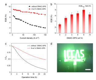
Fig. 4 (a) EQE-current density characteristics of LECs with 8 wt% and without DMAC-DPS. (b) EQE values measured at 100 cd m $^{-2}$  and different sensitizer concentrations. (c) Normalized luminance as a function of operational time with an initial of  $L_0=100$  cd m $^{-2}$  at constant current with 8 wt% and without DMAC-DPS. (d) Image of TSF-LECs with a pattern of the abbreviation of "ICCAS", and the scale bar represents 0.5 cm.
