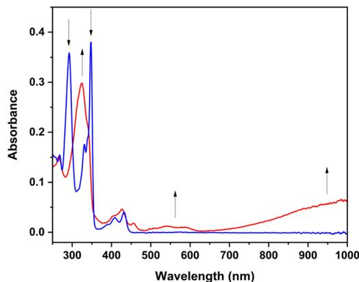
Fig. 9 UV-Vis absorption spectral changes resulting from oxidation of  $m\text{-ICz-Br}$  (blue) to  $[m\text{-ICz-Br}]^+$  (red.). Conditions: in  $\text{CH}_2\text{Cl}_2/\text{Bu}_4\text{NPF}_6$  at  $T = 298$  K; Pt minigrad in an OTTLE cell.
