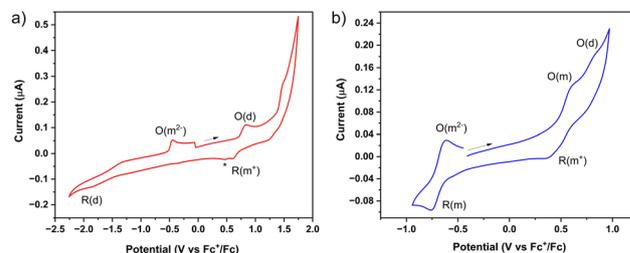
**Fig. 8** Cyclic voltammograms of (a) 0.2 mM (*m*-ICz-CN)<sub>2</sub> in CH<sub>2</sub>Cl<sub>2</sub>/Bu<sub>4</sub>NPF<sub>6</sub> at 293 K;  $\nu = 100 \text{ mV s}^{-1}$ , Pt disk microelectrode, and (b) ca. 0.2 mM *m*-ICz-CN in *o*-dichlorobenzene/Bu<sub>4</sub>NPF<sub>6</sub> at 393 K;  $\nu = 100 \text{ mV s}^{-1}$ , Pt disk microelectrode. Abbreviations: d = dimer (*m*-ICz-CN)<sub>2</sub>, m = monomer *m*-ICz-CN, O = oxidation, R = reduction.
