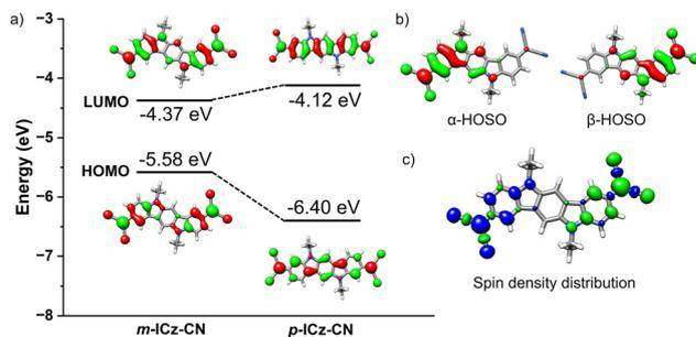
Fig. 3 (a) DFT-calculated (M06-2X/6-31G\*\*) molecular orbital diagram of *m*-ICz-CN and *p*-ICz-CN. (b) Calculated highest-occupied single orbitals (HOSO) of α and β electrons for *m*-ICz-CN. (c) Spin density distribution in the diradical singlet ground state of *m*-ICz-CN at the (U)M06-2X/6-31G\*\* level of theory with an isosurface value of 0.03 a.u. The blue and green surfaces represent α and β spin densities, respectively.
