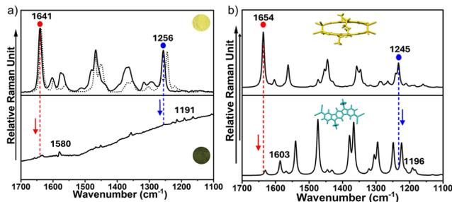
Fig. 13 (a) Top: FT-Raman spectra at  $\lambda_{\text{exc}} = 1064$  nm of the yellow powder of  $(m\text{-ICz-CN})_2$  (black line) and its brominated precursor  $m\text{-ICz-Br}$  (black dots). Bottom: Raman spectrum at  $\lambda_{\text{exc}} = 785$  nm of isolated diradical  $m\text{-ICz-CN}$  in the solid state at 410 K. (b) Theoretical Raman spectra of  $(m\text{-ICz-CN})_2$  (top) and  $m\text{-ICz-CN}$  (down) at the M06-2X/6-31G\*\* level.
