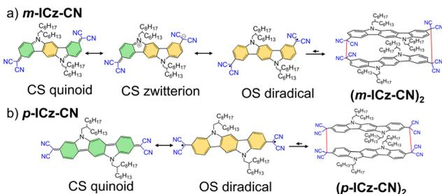
Fig. 1 Structures of (a) ***m*-ICz-CN** and (b) ***p*-ICz-CN** open-shell (OS) diradicals and their closed-shell (CS) quinoid/zwitterion resonance structures. The cyclophane dimeric arrangements of (a) ***m*-ICz-CN** and (b) ***p*-ICz-CN** are also shown.
