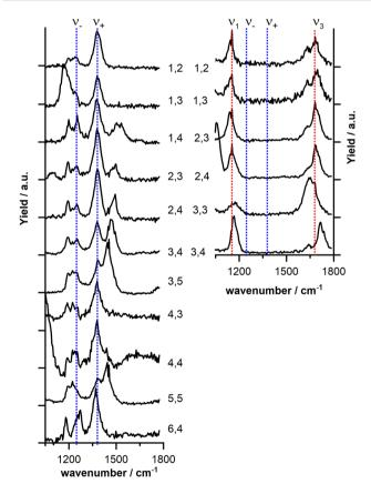
Fig. 2 IR-MPD spectra of (left column) cationic  $Cu_xO_v(CO_2)^+$  and (right column) anionic  $Cu_xO_y(CO_2)^-$  complexes (labeled x,y). The blue dotted lines indicate the Fermi dyad and the red dotted lines modes of activated CO2. The black tick marks on the y-axis indicate the zero depletion yield for each spectrum. The spectra of the anionic complexes were recorded at reduced IR laser fluence (cf. Section 2.1)
