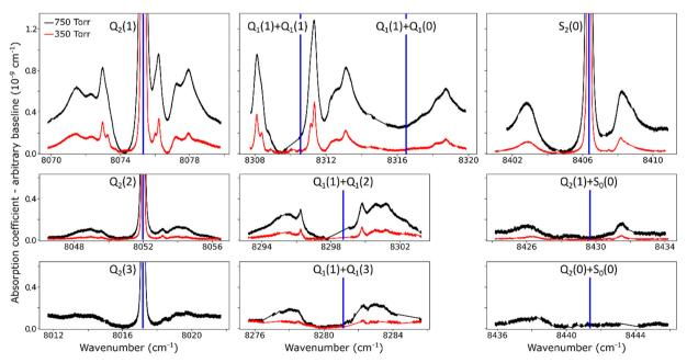
Fig. 4 Close-up view of dimer structures observed at room temperature around H<sub>2</sub> monomer lines and simultaneous transitions, at 350 Torr (red) and 750 Torr (black). Some spectral gaps are observed due to strong absorption lines of water vapor. Calculated positions of monomer resonances are indicated by blue vertical lines. The same relative spectral scale and the same intensity scale are used for the different panels. An empirical linear baseline was subtracted from each spectrum
