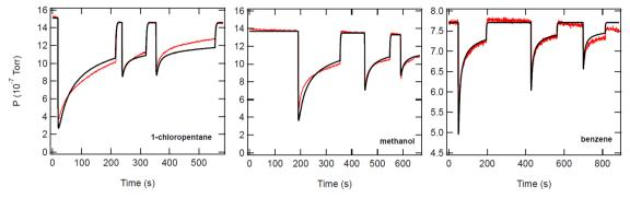
Fig. 10 Kinetic multilayer model simulations for uptake profiles of 1-chloropentane, methanol and benzene on silica at 170 K. The experimental data are shown in red, and the model fit is shown in black. The fitted parameters are  $D_{g,p} = 0.0015$  cm<sup>2</sup> s<sup>-1</sup>, 0.0012, 0.001 and  $k_d = 0.1$ , 0.4, and 3 s<sup>-1</sup> for 1-chloropentane, methanol, and benzene respectively.
