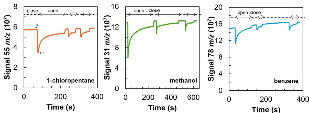
**Fig. 2** Representative uptake profiles of 1-chloropentane, methanol, and benzene on silica particles at 170 K. Initial chamber pressures were  $0.9 \times 10^{-5}$ ,  $1.5 \times 10^{-5}$ , and  $1.6 \times 10^{-5}$  torr for 1-chloropentane, methanol, and benzene, respectively.
