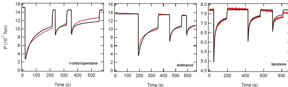
**Fig. 10** Kinetic multilayer model simulations for uptake profiles of 1-chloropentane, methanol and benzene on silica at 170 K. The experimental data are shown in red, and the model fit is shown in black. The fitted parameters are  $D_{g,p} = 0.0015 \text{ cm}^2 \text{ s}^{-1}$ , 0.0012, 0.001 and  $k_d = 0.1$ , 0.4, and  $3 \text{ s}^{-1}$  for 1-chloropentane, methanol, and benzene respectively.
