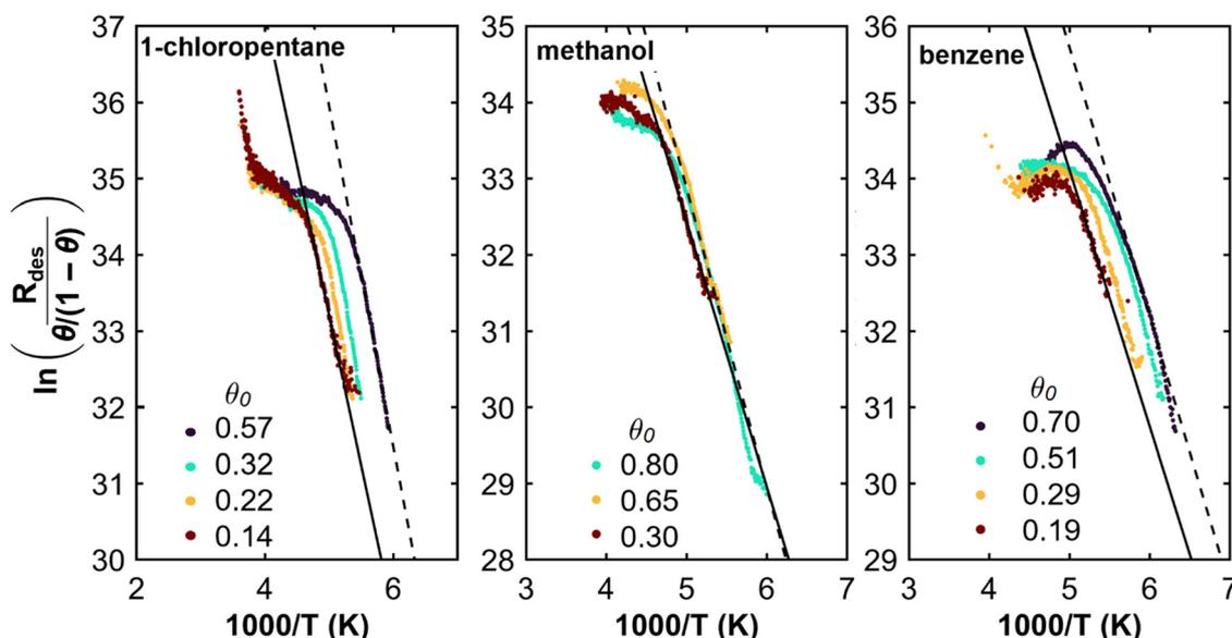
Fig. 8 Natural logarithms of desorption rates divided by  $\theta/(1-\theta)$  for 1-chloropentane, methanol, and benzene (from left to right). The slopes of the curves are equal to  $E_d/R$ . In each panel the dashed curve is the best fit to the largest initial coverage and the solid curve is the best fit to the lowest initial coverage.
