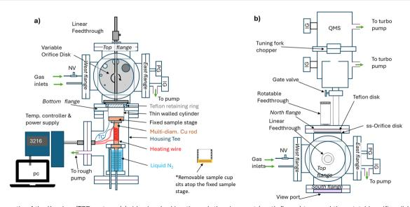
Fig. 1 Schematic of the Knudsen/TPD system: (a) side view looking through the view port (south flange) to reveal the rotatable orifice disk facing the north flange. (b) Top view of cell with line to mass spectrometer. PG = pressure gauge, IG = ionization gauge, TC = thermocouple, NV = needle valve, QMS = quadrupole mass spectrometer
