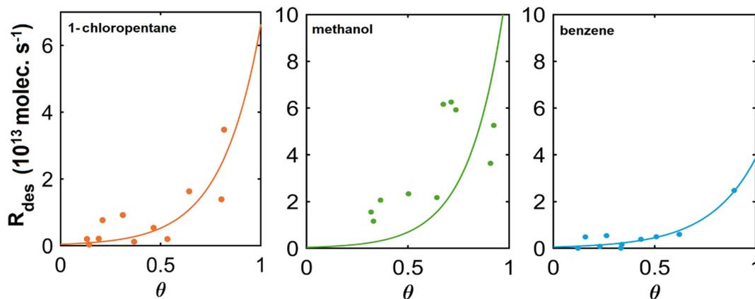
Fig. 7 Desorption rates at 170 K were determined from the TPD curves with varying initial coverages. The surface coverage at the specified temperature was determined by integration of the TPD curves. The solid curves are the best fit to the data.
