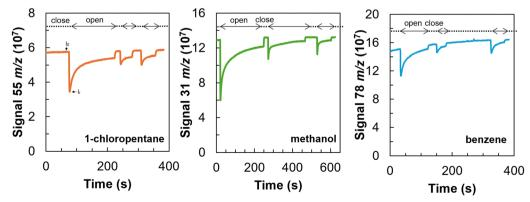
Fig. 2 Representative uptake profiles of 1-chloropentane, methanol, and benzene on silica particles at 170 K. Initial chamber pressures were  $0.9 \times 10^{-5}$ .  $1.5 \times 10^{-5}$ , and  $1.6 \times 10^{-5}$  torr for 1-chloropentane, methanol, and benzene, respectively
