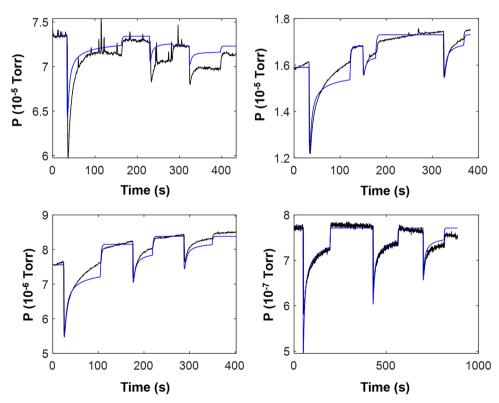
Fig. 9 Measurements (black) and kinetic multilayer model simulations (blue) of benzene uptake on silica particles for different initial benzene pressures.
