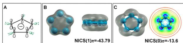
Fig. 3 (A) Atomic orbital diagram of the  $\text{cyclo-N}_5^-$  anion; (B) top and side views of the LDOS isosurface at the lowest energy level of the aromatic  $\pi$ -system; (C) LDOS isosurface at the lowest energy level of the aromatic  $\sigma$ -system. Reproduced with permission from ref. 91. Copyright 2019, Wiley.
