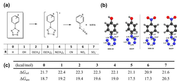
Fig. 1 (a) Schematic view for the decomposition of arylpentazoles with substituents **0–7**; (b) selected geometries of transition state structures; (c) reaction barriers of decomposition of *para*-substituted arylpentazoles **0–7**. Reproduced with permission from ref. 72. Copyright 2019, The Royal Society of Chemistry.
