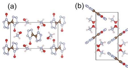
Fig. 7 Crystal structure of TKX-50. Panel (a) is the view from the *a* direction, and panel (b) is the view from the *c* direction. Reproduced with permission from ref. 104. Copyright 2014, American Chemical Society.
