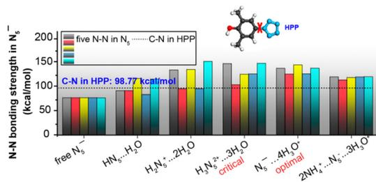
Fig. 5 N–N bond strengths in the *cyclo*-N<sub>5</sub><sup>−</sup> anion at various acid concentrations with respect to the C–N bond strength in HPP (dashed line). Reproduced with permission from ref. 90. Copyright 2019, American Chemical Society.
