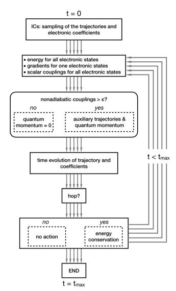
Fig. 5 Schematic representation of the SHXF algorithm, with all the gray arrows (5 in this case, so as to indicate the propagation of 5 physical trajectories) being represented as thin lines, since all the associated tasks can be performed trivially in parallel.
